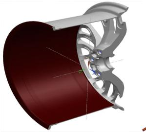
• Chrome wheels with a coated barrel (areas illustrated in red), refinishing is possible. However, the required refinishing process cannot be performed in the dealer environment. Refer to Refinisher's Responsibility – Outside Company later in this bulletin.
