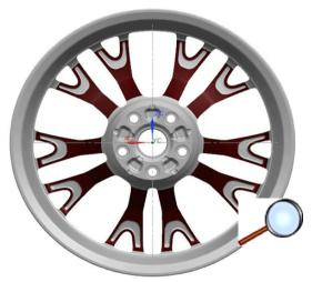
• Rear of the spoke or drop well on the rear of the hub (areas illustrated in red), refinishing is possible. However, the required refinishing process cannot be performed in the dealer environment. Refer to Refinisher's Responsibility – Outside Company later in this bulletin.
