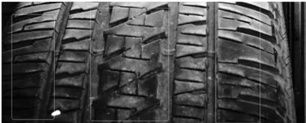
Figure 1: Full Tread View – “NORMAL” Tyre “Feathering” Wear on the Shoulder/Adjacent/Center Ribs
