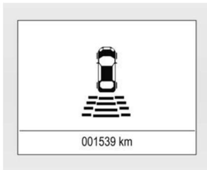
Additionally, the distance to rear objects is displayed by changing distance lines in the Driver Information Centre (DIC). The distance indication can be inhibited by vehicle messages with a higher priority. After dismissing the message, distance indication appears again if applicable.
