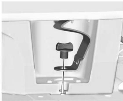
1. Turn the wing nut on the right-hand side and remove. This will also disconnect the load floor cover strap.
