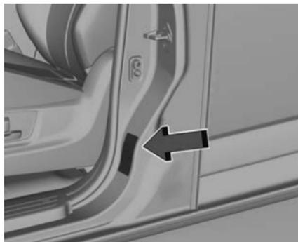
The correct pressures for tyres are shown on the tyre placard on the front passenger door frame and also in the tyre pressure table. See *Tyre Pressure* ⇨ 313.
