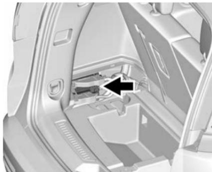
To access the fuse block, remove the underfloor storage tray. See *Cargo Management System* ⇨ 76.
