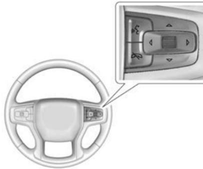
△ or ▽ : Turn the thumbwheel to move up or down in a list.
