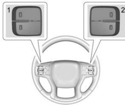
Infotainment system favourite and volume switches are on the back of the steering wheel.
