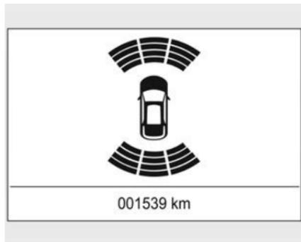
The system warns the driver with a visual display in the Driver Information Centre (DIC), acoustic signals and/or, if equipped and enabled, may pulse the driver's seat when potentially hazardous objects are detected.
