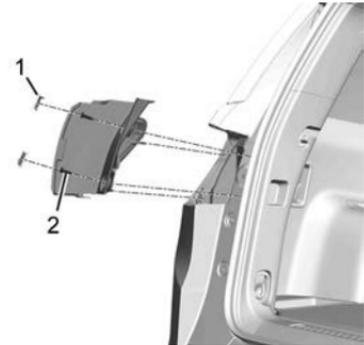
2. Carefully prise off the two screw covers (1) and remove the two screws (2).
