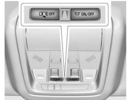
The dome lamp is in the overhead console.
