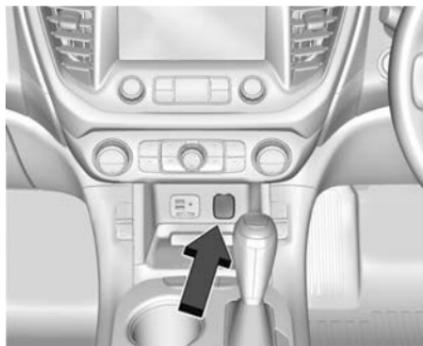
The front power outlet is located at the front of the centre console, below the climate controls.
