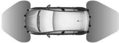
The system uses ultrasonic parking sensors located in the rear and front bumpers.
