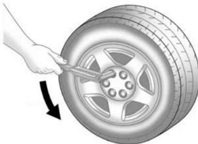
3. Turn the wheel wrench anticlockwise to loosen all the wheel nuts, but do not remove them yet.
