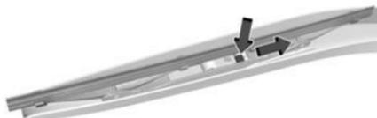
2. Push the release lever to disengage the hook and push the wiper arm toward the centre of the vehicle and out of the blade assembly.
