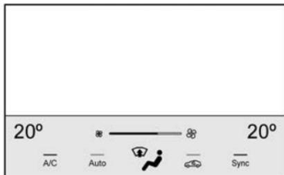
The climate control status display appears briefly when the instrument panel climate controls are adjusted.
