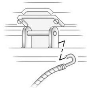
5. Hook the cable onto the outside portion of the liftgate hinges.
