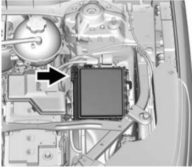
To remove the fuse block cover, press the clips on the cover and lift it straight up.
