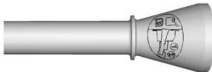
1. The capless funnel adapter is located with the vehicle tools/jack beneath the rear cargo area underfloor storage tray. See *Cargo Management System* ⇨ 76.
