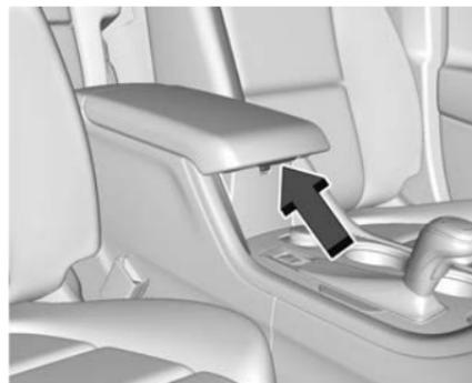
The centre console has a storage compartment under the armrest. Pull up the latch and lift to open.
