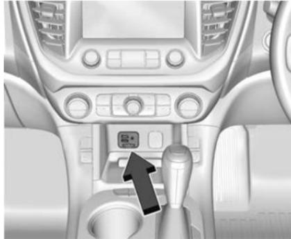
The vehicle has an auxiliary input jack located at the front of the centre console. Possible auxiliary audio sources include:
