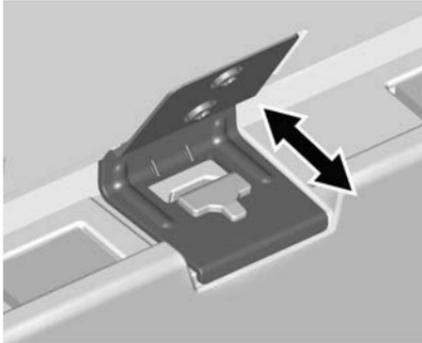
3. Disengage the load floor cover hinges by sliding rearward from the underfloor storage tray.
