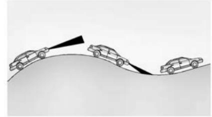
Do not use ACC when driving on hills or when towing a trailer.
