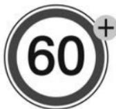
The current valid speed limit is displayed permanently in the lower line of the DIC (Type 1) or upper left of the instrument cluster (Type 2). If a speed sign with an add-on sign is detected, a + symbol is also displayed.
