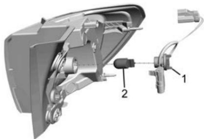
5. Remove the bulb socket (1) from the tail lamp assembly by turning it anticlockwise.
