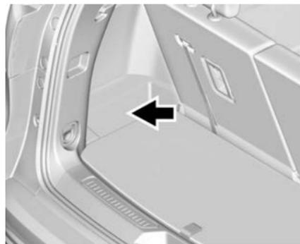
The rear fuse panel is located below the left-hand side trim panel in the rear compartment.
