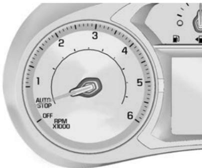
An Auto Stop is indicated by the tachometer needle moving to the AUTO STOP position. Once the engine restarts, the engine speed indication is resumed.
