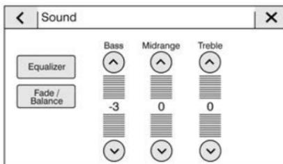
**Equaliser** : Touch to adjust Bass, Midrange and Treble using the controls on the infotainment display.
