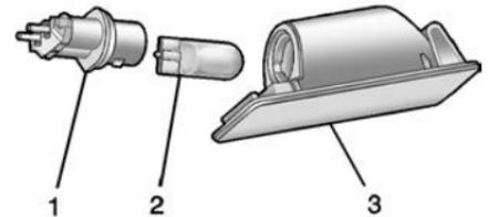
3. Remove the bulb socket (1) from the lamp assembly (3) by turning anticlockwise.
