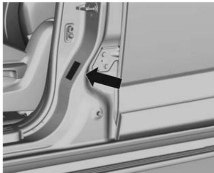
The vehicle compliance label is located on the front passenger's door frame.
