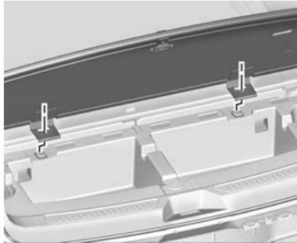
4. Lift the load floor cover up and remove. Place the cover in a safe location.
