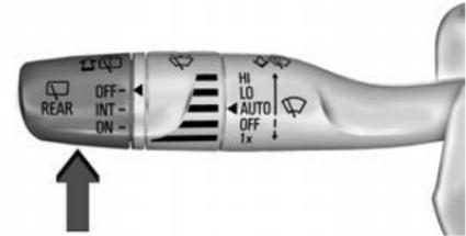
Turn the end of the windscreen wiper lever to operate the rear window wiper/washer.
