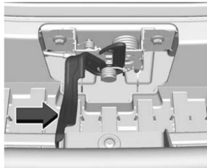
2. At the front of the vehicle, pull up on the centre of the bonnet slightly, and push the secondary bonnet release to your right.
