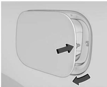
The fuel filler is behind the fuel door on the passenger side of the vehicle.
