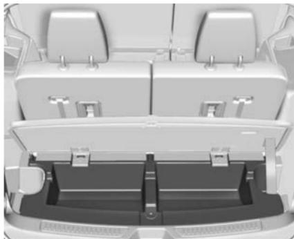
Raise the load floor cover to access the underfloor storage tray.
