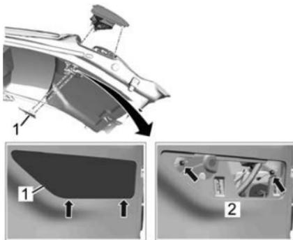
2. Carefully prise the lower portion of the liftgate access cover (1) at two places and remove the cover.
