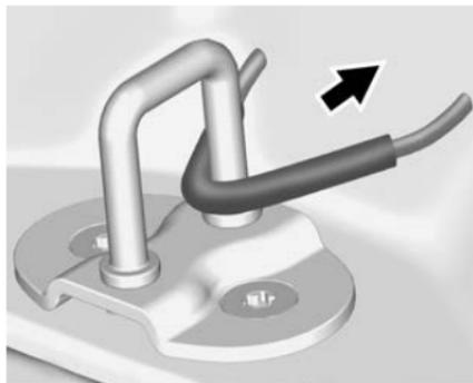
8. Make sure the metal tube is centred at the striker. Push the tube toward the front of the vehicle.
