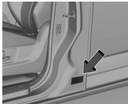
An identification label is located on the lower portion of the front passenger's door frame. The label shows the Vehicle Built Date and VIN.
