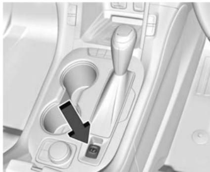
The Electric Parking Brake (EPB) switch is located on the centre console and can always be activated, even if the ignition is off.
