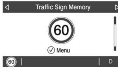
Traffic sign assistant recognises designated traffic signs via the front camera located behind the windshield in front of the interior rear view mirror, and displays the detected speed limit in the Driver Information Centre (DIC). Additionally, speed limit information from the navigation system map database may be utilised.
