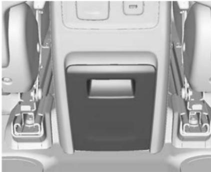
A storage bin is located at the rear of the centre console. Lift the handle up and slide the bin out.
