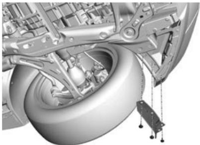
2. Remove the three screws and remove the front air deflector.
