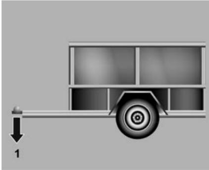
A trailer hitched to a vehicle places a weight on the tow bar. This weight is called the tow bar ball weight or tow ball load (1).
