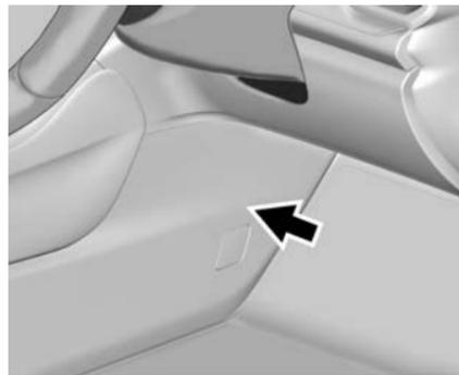
The instrument panel fuse block is inside the centre console on the right-hand side of the vehicle.
