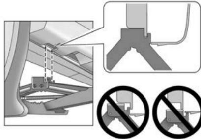
6. Turn the wheel wrench clockwise to raise the jack lift head until the slots in the jack head fit into the metal flange behind the cut out on the plastic moulding. Do not raise the vehicle yet.
