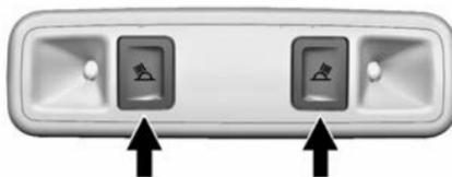
Press the buttons to turn the rear reading lamps on or off.
