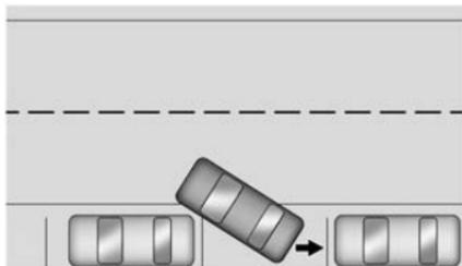
Follow the displayed instructions. When instructed to drive in reverse, shift to R (Reverse) to engage automatic steering. The steering wheel will briefly vibrate as a reminder to remove hands from the steering wheel.
