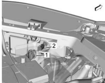
2. Remove the green bulb socket (1) from the headlamp assembly by turning it anticlockwise.
