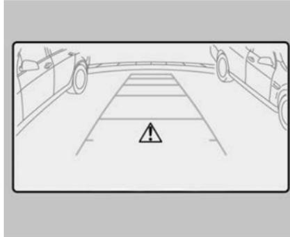
When the camera image is displayed, dynamic guidelines are also displayed to assist with reversing the vehicle.
