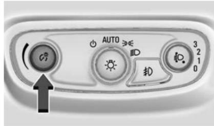
The brightness of the instrument panel lighting and steering wheel controls can be adjusted.
