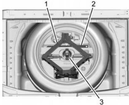
4. Turn the wing nut (3) anticlockwise to remove the jack (1) and wheel wrench (2). Place the tool container near the tyre being changed.
