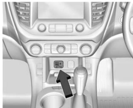
The front USB port is located at the front of the centre console, below the climate controls. It contains two outlets which can be used to charge USB devices and also to connect an audio device to the infotainment system. See *USB Port* ⇨ 135.
