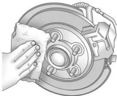
11. Remove any rust or dirt from the wheel bolts, mounting surfaces, and spare wheel.
