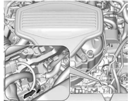
The engine serial number is located on the vehicle front side of the engine block.
