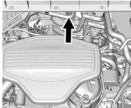
The VIN is also stamped in the engine compartment on the firewall. It is also included on the vehicle compliance label.
