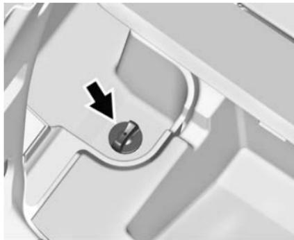
2. Turn the wing nut on the left-hand side and remove.
