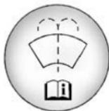
Open the cap with the washer symbol on it. Add washer fluid until the tank is full. See *Engine Compartment Overview* ⇨ 258 for reservoir location.
