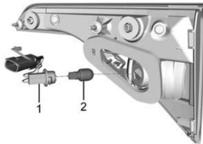
5. Remove the bulb socket (1) from the tail lamp assembly by turning it anticlockwise.
