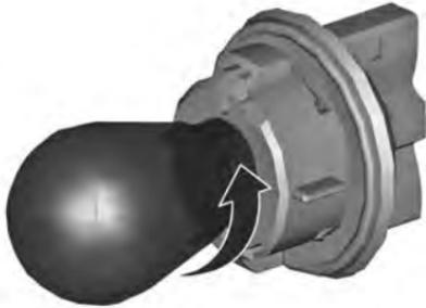
3. Remove the bulb from the socket by turning anticlockwise.
