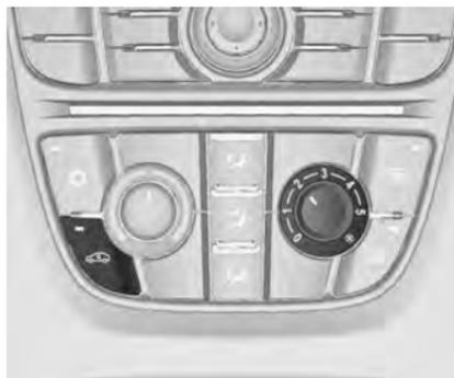
Press 🚗 to activate air recirculation mode. Activation is indicated by the LED in the button.
