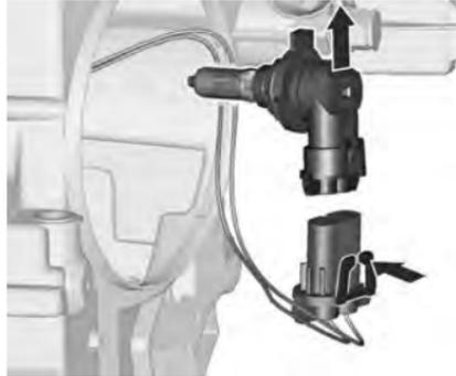
3. Disengage the bulb holder from the plug connector by pressing the retaining lug.
