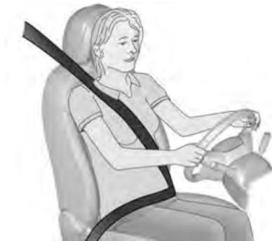
The seat belts are locked during heavy acceleration or deceleration of the vehicle holding the occupants in the sitting position. Therefore the risk of injury is considerably reduced.
