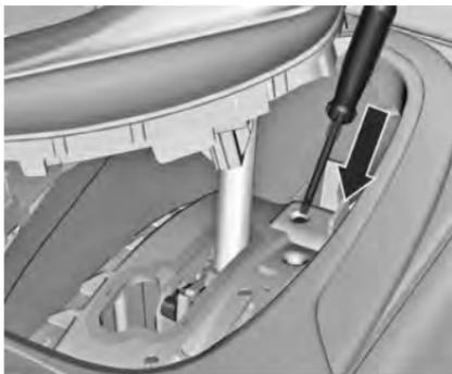
3. Insert a screwdriver into the opening as far as it will go and move the selector lever out of **P** or **N**. If **P** or **N** is engaged again, the selector lever will be locked in position again. Have the cause of the power supply interruption remedied by a Holden dealer.
