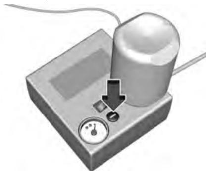
If the prescribed tyre pressure is not obtained within 10 minutes, remove the tyre repair kit. Move the vehicle one tyre rotation. Reattach the tyre repair kit and continue the filling procedure for 10 minutes.
