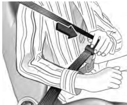
Withdraw the belt from the retractor, guide it untwisted across the body and insert the latch plate into the buckle. Tighten the lap belt regularly whilst driving by pulling the shoulder belt.
