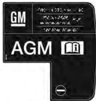
An AGM battery can be identified by the label on the battery. We recommend the use of an original Holden vehicle battery.
