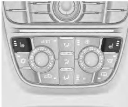
Adjust heating to the desired setting by pressing
