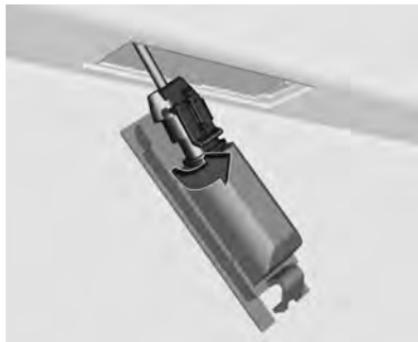
2. Remove lamp downwards, taking care not to pull on the cable.
