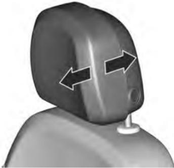
To adjust horizontally, pull the lower front portion of the head restraint forwards. It engages in several positions.
