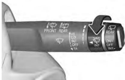
Turn the adjuster wheel to adjust the sensitivity:
