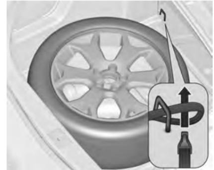
2. Place the loop end of the strap through the front lashing eye on the appropriate side.
