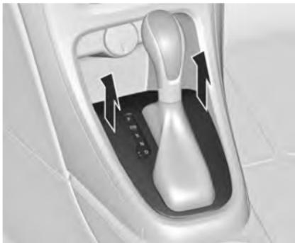
2. Release the selector lever trim from the centre console at the front, fold it upwards and rotate it to the left.
