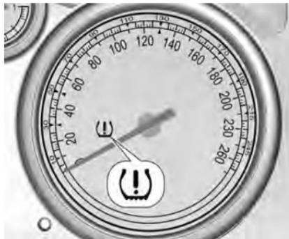
A detected low tyre pressure condition is indicated by the control indicator
