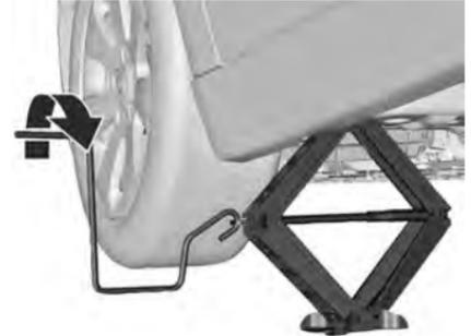
Attach jack handle and with the jack correctly aligned rotate handle until wheel is clear of the ground.
