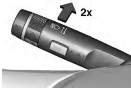
Intelligent light ranging and automatic high beam activation are switched on together by pushing the indicator lever twice. They can be switched on with ignition on.
