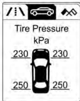
Turn the adjuster wheel to select the tyre pressure monitoring system.
