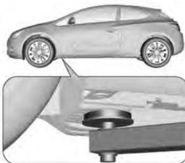
Front arm position of the lifting platform at the underbody.
