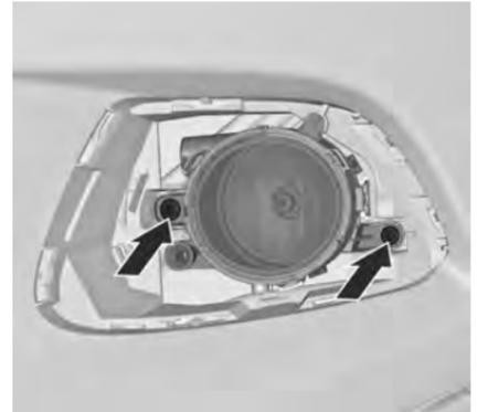
2. Unscrew both screws and remove light assembly from the bumper.
