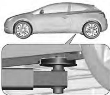
Rear arm position of the lifting platform centrally under the recess of the sill.
