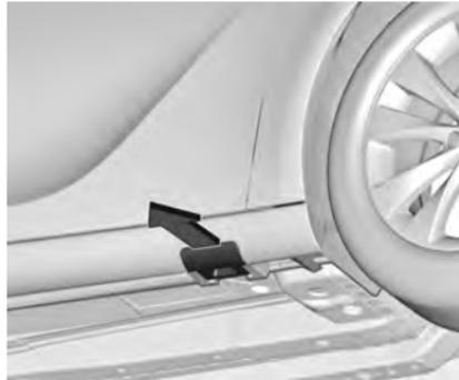
Some versions have sill panellings with covered vehicle jacking points: pull out the cover at the respective jacking point firstly.
