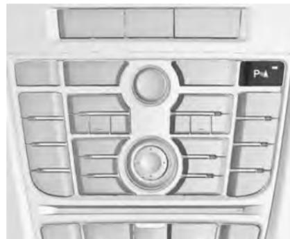
An illuminated LED in the parking assist button **P** with a warning triangle indicates that the system is ready to operate.
