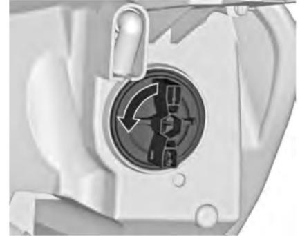
1. Rotate bulb socket (2) anticlockwise to disengage. Withdraw the bulb socket from the reflector.
