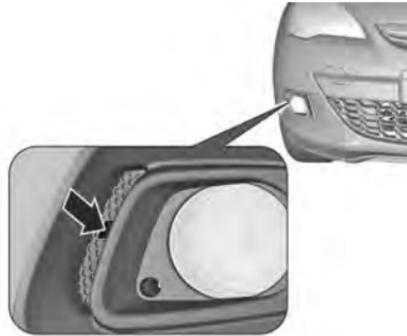
1. Disengage the cover with a screwdriver in the recess and remove the cover.
