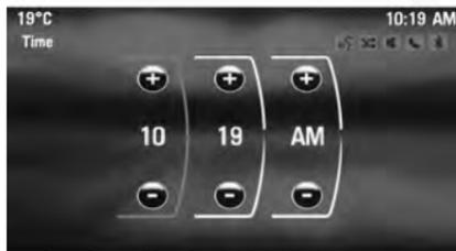
Push the multifunction knob outer ring to confirm the input. The coloured background moves to the next setting.
