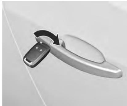
Manually unlock the driver's door by turning the key in the lock. Switch on the ignition and press the central locking button
