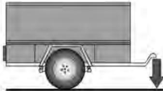
When a trailer is hitched to the vehicle, it places a weight on the tow bar. This weight is called the 'tow ball load'.
