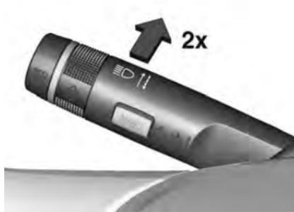
The high beam assist is activated by pushing the indicator lever twice with a speed above 40 km/h.
