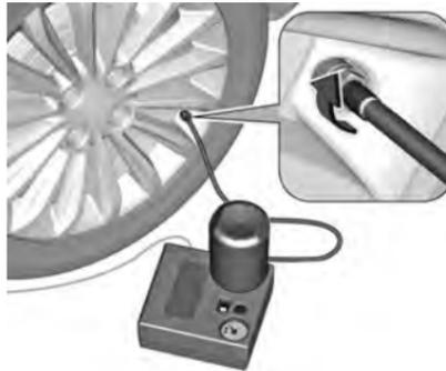
6. Unscrew valve cap from defective tyre.
