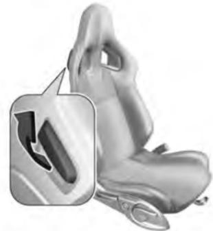
The illustration shows the release lever on VXR seat.
