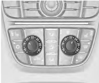
If the minimum temperature **Lo** is set, the climate control system runs at maximum cooling, if cooling
