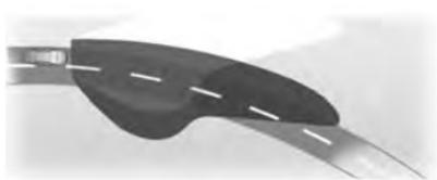
The light beam pivots based on steering wheel angle and speed, improving lighting in curves.
