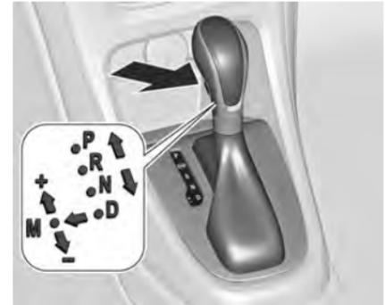
**P** : park position, press release button, wheels are locked, engage only when the vehicle is stationary and parking brake is applied
