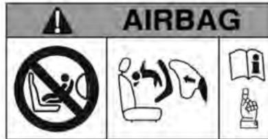
There is a warning label on the side of the instrument panel, visible when the front passenger door is open, or on the front passenger sun visor.
