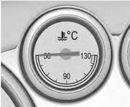
Displays the coolant temperature.
