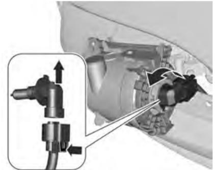
3. Turn the bulb socket anti-clockwise and remove it from the reflector.
