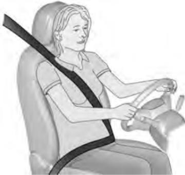
The seat belts are locked during heavy acceleration or deceleration of the vehicle holding the occupants in the sitting position. Therefore the risk of injury is considerably reduced.
