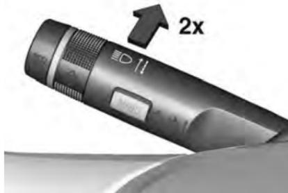
The high beam assist is activated by pushing the indicator lever twice with a speed above 40 km/h.
