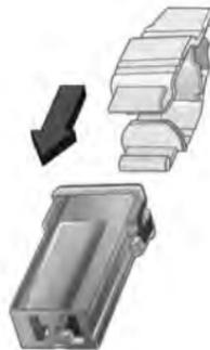
Place the fuse extractor on the various types of fuse from the top or side, and withdraw fuse.
