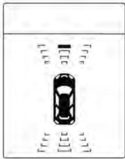
The distance to a front and rear obstacle is indicated by changing distance lines around the vehicle.
