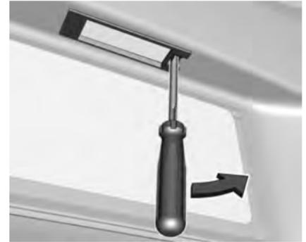
1. Insert screwdriver in recess of the cover, press to the side and release spring.
