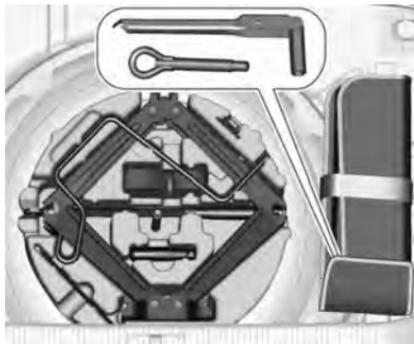
The jack, the tools and a strap for securing a damaged wheel are in the tool box below the spare wheel in the load compartment. The wheel wrench and the towing eye are in the tool bag located in the spare wheel well near the tool box. Spare wheel ↗ 238.
