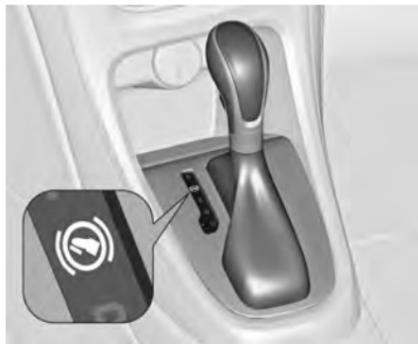
Without brake pedal applied, the control indicator
