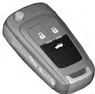
If equipped, pressing
