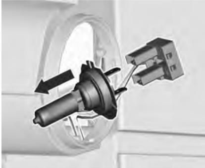
3. Disengage the bulb from the plug connector by pulling.
