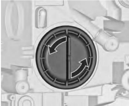
1. Rotate the cap (1) anticlockwise and remove it.
