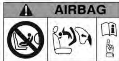
Additionally there is a warning label on the side of the instrument panel, visible when the front passenger door is open, or on the front passenger sun visor.
