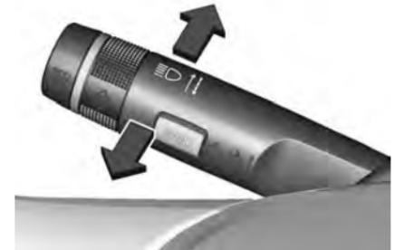
To switch from low to high beam, push lever.
