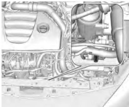
The engine serial number is located in the front part of the engine compartment.
