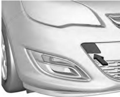
Insert a screwdriver in the slot at the lower part of the cap. Release the cap by carefully moving the screwdriver downwards.
