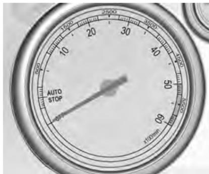
Displays the engine speed.
