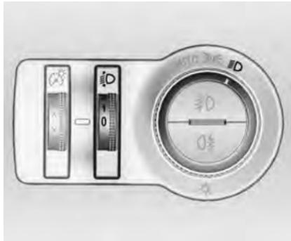
To adapt headlight range to the vehicle load to prevent dazzling: turn thumb wheel  $\text{D}$  to required position.
