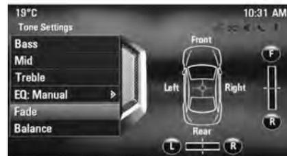
To adjust the volume distribution between the front and rear speakers in the vehicle, select **Fade**. Adjust the setting as desired.
