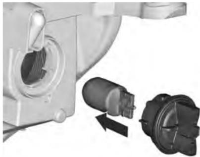
2. Remove the bulb from the socket by pulling.
