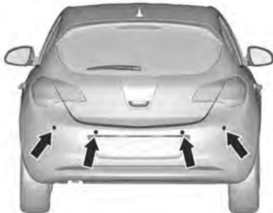
The system has four ultrasonic parking sensors in the rear bumper.
