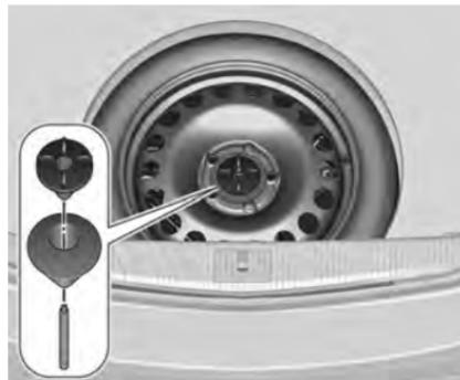
Position the excentric conus in the recess of the spare wheel before turning the wing nut right back.
