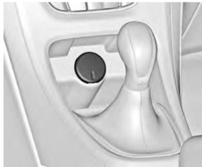
A 12 Volt power outlet is located in the front console.
