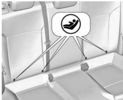
Fasten vehicle-approved ISOFIX child restraint systems to the ISOFIX mounting brackets. Specific vehicle ISOFIX child restraint system positions are marked in the table. ISOFIX mounting brackets are indicated by a label on the backrest.
