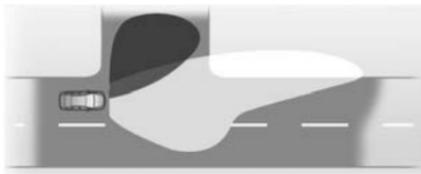
On tight bends or when turning off, depending on the steering angle or the turn signal light, an additional left or right reflector is switched on which illuminates the road at a right angle to the direction of travel. It is activated up to a speed of 40 km/h.
