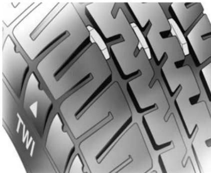
The legally permissible minimum tread depth (1.6 mm) has been reached when the tread has worn down as far as one of the tread wear indicators (TWI). Their position is indicated by markings on the sidewall.
