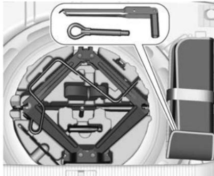
The jack, the tools and a strap for securing a damaged wheel are in the tool box below the spare wheel in the load compartment. The wheel wrench and the towing eye are in the tool bag located in the spare wheel well near the tool box. Spare wheel ⇨ 237.
