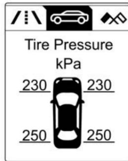
Turn the adjuster wheel to select the tyre pressure monitoring system. System status and pressure warnings are displayed by a message with the corresponding tyre flashing in the Driver Information Centre.
