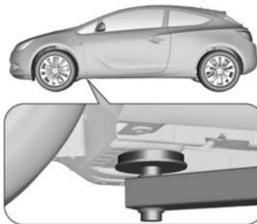
Front arm position of the lifting platform at the underbody.
