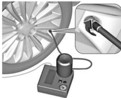
6. Unscrew valve cap from defective tyre.
