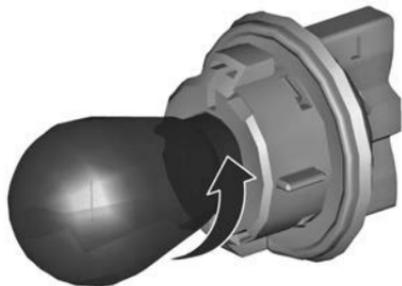
3. Remove the bulb from the socket by turning anticlockwise.
