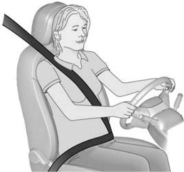
Pull out the seat belt and fasten in belt buckle. The seat belt must not be twisted and must fit close against the body. The backrest must not be tilted back too far (maximum approx. 25 °). To unfasten belt, press red button on belt buckle.
