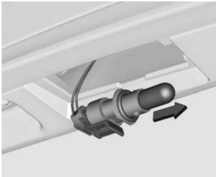
3. Remove bulb holder from lamp housing by turning anticlockwise.
