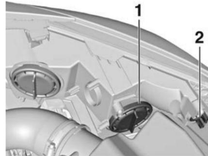
**Bi-Halogen Headlight (1)** with one bulb for low and high beam.
