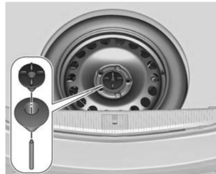
Position the excentric conus in the recess of the spare wheel before tightening the wing nut.
