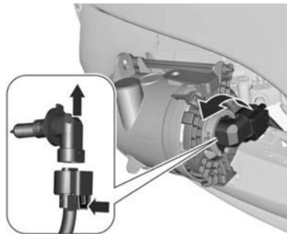
3. Turn the bulb socket anticlockwise and remove it from the reflector housing.
