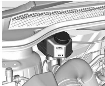
The brake fluid level must be between the **MIN** and **MAX** marks.
