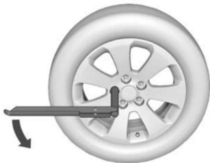
2. Fold out the wheel wrench and install ensuring that it locates securely and loosen each wheel nut by half a turn.
