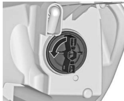
1. Rotate bulb socket (2) anticlockwise to disengage. Withdraw the bulb socket from the reflector.
