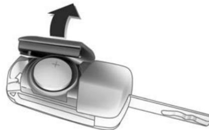
Extend the key and open the unit. Replace the battery (battery type CR 2032), paying attention to the installation position. Close the unit and synchronise.
