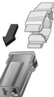
Place the fuse extractor on the various types of fuse from the top or side, and withdraw fuse.
