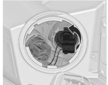
2. Rotate the bulb holder anticlockwise to disengage. Withdraw the bulb holder from the reflector.
