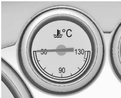
Displays the coolant temperature.
