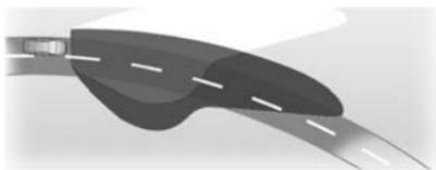
The light beam pivots based on steering wheel angle and speed, improving lighting in curves.
