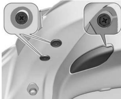
1. Open the tailgate and remove the covers on the respective side.
