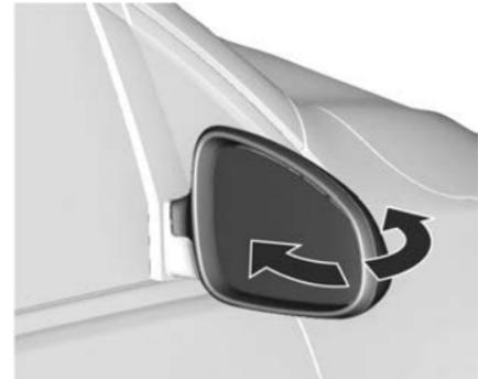
For pedestrian safety, the exterior mirrors will swing out of their normal mounting position if they are struck with sufficient force. Reposition the mirror by applying slight pressure to the mirror housing.
