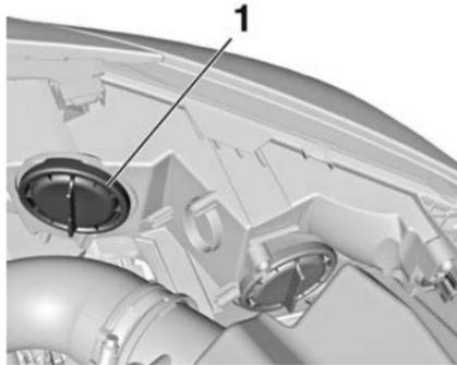
1. Rotate cap (1) anticlockwise and remove it.
