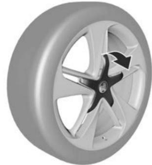
Alloy wheels with centre cap: Disengage centre cap by carefully pulling each side of the cap away from the wheel with your hands.
