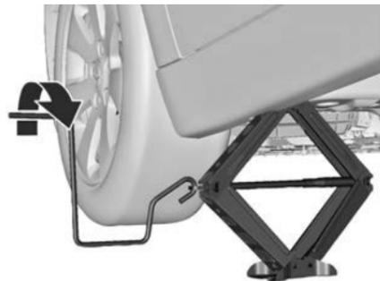
Attach jack handle and with the jack correctly aligned rotate handle until wheel is clear of the ground.
