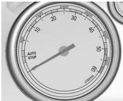
Displays the engine speed.
