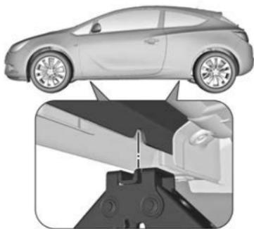
3. Ensure the jack is correctly positioned under the relevant vehicle jacking point.
