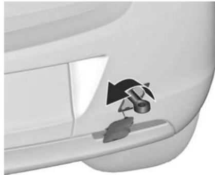
Screw in the towing eye as far as it will go until it stops in a horizontal position.
