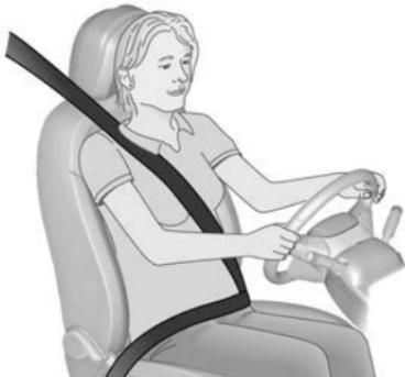
The seat belts are locked during hard acceleration or deceleration of the vehicle holding the occupants in the seated position. Therefore the risk of injury is considerably reduced.
