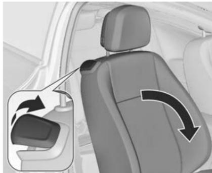
Lift release lever and fold backrest forwards. Slide seat forwards.
