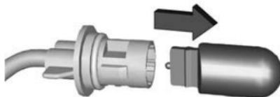
3. Pull bulb from bulb holder and replace it.
