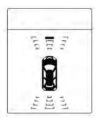
The distance to a front and rear obstacle is indicated by changing distance lines around the vehicle.
