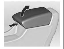
Press button to fold up the armrest. The armrest must be in rearmost position.
