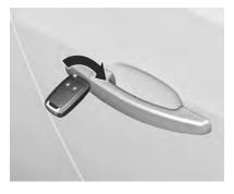
Manually unlock the driver's door by turning the key in the lock. Switch on the ignition and press the central locking button at to unlock the other doors, tailgate and fuel filler flap.
