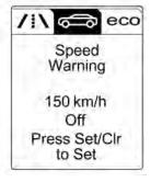
Speed Warning: if exceeding the preset speed, a warning chime will be activated
