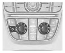
Press to switch on cooling.
