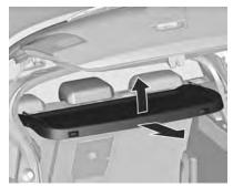
Lift cover at the rear and push it upwards at the front.
