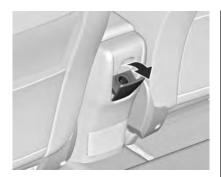
A further 12 Volt power outlet may be located in the rear console. Fold the cover downwards.
