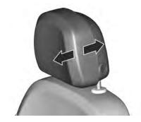
To adjust horizontally, pull the lower front portion of the head restraint forwards. It engages in several positions.
