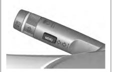
Press **MENU** to switch between the menus or to return from a submenu to the next higher menu level.
