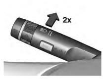
The high beam assist is activated by pushing the indicator lever twice with a speed above 40 km/h.
