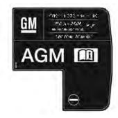
An AGM battery can be identified by the label on the battery. We recommend the use of an original Holden vehicle battery.
