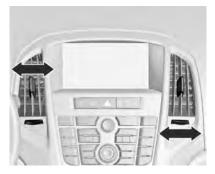
To open the vent, turn the adjuster wheel towards the bigger ■ symbol. Adjust the air amount at the vent outlet by turning the adjuster wheel.
