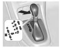
P: park position, press release button, wheels are locked, engage only when the vehicle is stationary and parking brake is applied
