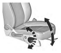
Lever pumping motion up : front end higher
