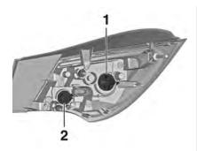
5. Remove the bulb holder by turning and replace the bulb by withdrawing or pushing the bulb slightly into the socket and rotating anticlockwise:
