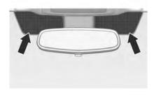
The marked areas on the windscreen are not covered with the coating. Devices for electronic data recording and fee payment must be attached in these areas. Otherwise data recording malfunctions may occur.
