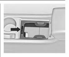
Press button to remove the frame of the cupholder. The frame can be stowed in the glovebox.
