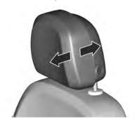
To adjust horizontally, pull the lower front portion of the head restraint forwards. It engages in several positions.
