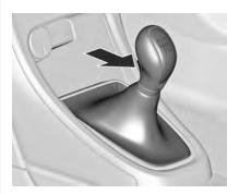
To engage reverse, with the vehicle stationary wait 3 seconds after depressing the clutch pedal and then press the release button on the selector lever and engage the gear.
