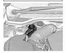
Power steering fluid level normally does not have to be checked. If an unusual noise sounds during steering or the power steering reacts unusually, seek the assistance of a Holden dealer.
