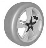
Alloy wheels with centre cap: Disengage centre cap by carefully pulling each side of the cap away from the wheel with your hands.
