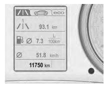
The bottom line displays the recorded distance in km.
