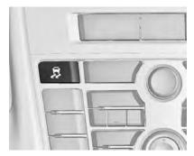
For very high-performance driving ESC and TC can be deactivated separately. The following modes are selectable:
