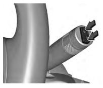
Press the rocker switch to activate the rear window wiper:
