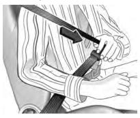
Withdraw the belt from the retractor, guide it untwisted across the body and insert the latch plate into the buckle. Tighten the lap belt regularly whilst driving by pulling the shoulder belt
