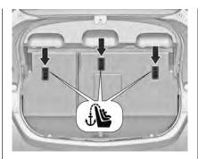
The fastening eyes are on the backside of rear seats.
