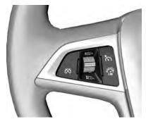
With automatic transmission, only activate cruise control in automatic mode.
