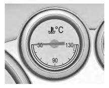
Displays the coolant temperature.
