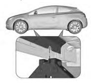
Ensure the jack is correctly positioned under the relevant vehicle jacking point.
