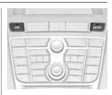
VXR Flex Ride driving system allows the driver to select between three driving modes:
