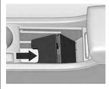
A further storage compartment is located under the intermediate shelf. Fold up the intermediate shelf and fix it in the vertical position. The frame of the cupholder can be reintegrated to stow bottles.
