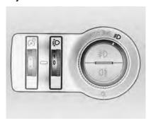
To adapt headlight range to the vehicle load to prevent dazzling: turn thumb wheel position.
