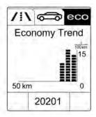
e Economy Trend: Displays the average consumption development over a distance of 50 km. Filled segments display the consumption in 5 km steps and shows the effect of topography or driving behaviour on fuel consumption.
