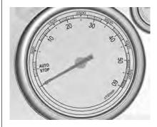
Displays the engine speed.
