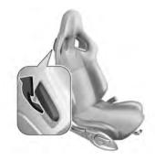
The illustration shows the release lever on VXR seat.
