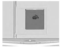
The closed cover can be secured from the side of the load compartment. Turn the knob 90°:
