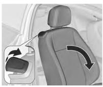
Lift release lever and fold backrest forwards. Slide seat forwards.
