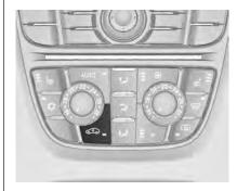
Press to activate the air recirculation mode. Activation is indicated by illumination of the LED in the button.
