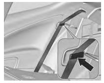
Take the seat belt out of the seat backrest guide and put it behind the retainer as shown in the illustration.
