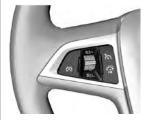
Press @. If cruise control has been activated before, it is switched off when speed limiter is activated and the control indicator (5) extinguishes.
