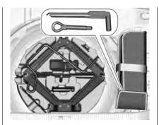
The jack, the tools and a strap for securing a damaged wheel are in the tool box below the spare wheel in the load compartment. The wheel wrench and the towing eye are in the tool bag located in the spare wheel well near the tool box. Spare wheel ▷ 238.
