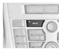
Deactivate the stop-start system manually by pressing **eco**.
