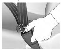
To release belt, press red button on belt buckle.
