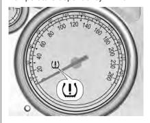
A detected low tyre pressure condition is indicated by the control indicator  $\textcircled{1} \Rightarrow 71$ .
