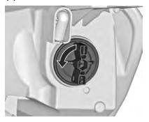
Rotate bulb socket (2)
