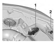
**Bi-Halogen Headlight (1)** with one bulb for low and high beam. **Sidelight/Daytime running light (2)**.
