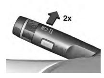
Intelligent light ranging and automatic high beam activation are switched on together by pushing the indicator lever twice. They can be switched on with ignition on.
