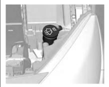
Fill with clean water mixed with a suitable quantity of windscreen washer solution.
