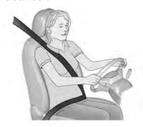
Pull out the seat belt and engage in belt buckle. The seat belt must not be twisted and must fit close against the body. The backrest must not be tilted back too far (maximum approx. 25°).
