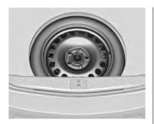
The spare wheel is located in the load compartment beneath the floor covering. It is secured with a wing nut. To remove:
