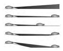
A special topographical evaluation function detects preceding vehicles on hills or slopes by recognising the rear light moving ahead. The system adjusts the height of the light range to ensure optimum illumination on the road ahead without dazzling.
