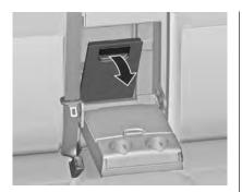
• Pull the grip and open the cover. Suitable for loading long, narrow objects.
