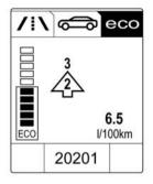
Shift indication: Current gear is indicated inside an arrow. The figure above recommends upshifting for fuel saving reasons.
