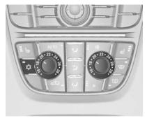
Press to switch on cooling. The LED in the button illuminates to indicate activation. Cooling is only functional when the engine is running and climate control fan is switched on.
