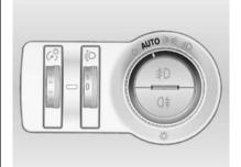
When the automatic light control function is switched on and the engine is running, the system switches between daytime running light and headlights automatically depending on the lighting conditions and information given by the rain sensor system.
