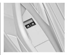
Operate the switch for the respective window by pushing to open or pulling to close.
