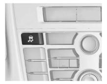
For very high-performance driving ESC and TC can be deactivated separately. The following modes are selectable:
