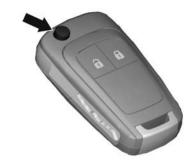
Press button to extend. To fold the key, first press the button.
