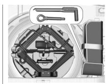
The jack, the tools and a strap for securing a damaged wheel are in the tool box below the spare wheel in the load compartment. The wheel wrench and the towing eye are in the tool bag located in the spare wheel well near the tool box. Spare wheel ▷ 237.
