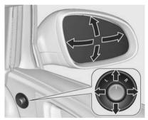
Select the relevant exterior mirror by turning the control to left **(L)** or right **(R)**. Then swivel the control to adjust the mirror.
