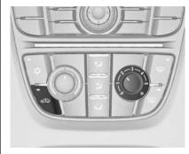
Press \$\sigma\$ to activate air recirculation mode. The LED in the button illuminates to indicate activation.
