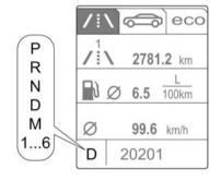
The mode or selected gear is shown in the transmission display.
