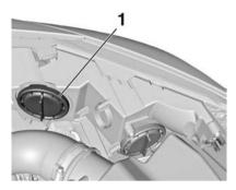
Rotate cap (1) anticlockwise and remove it.
