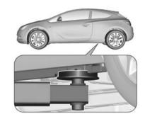
Rear arm position of the lifting platform centrically under the recess of the sill.
