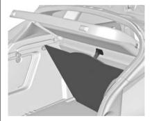
The rear floor cover can be lifted. Hang the loop on the hook on the lower side of the load compartment cover.
