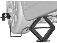
Attach jack handle and with the jack correctly aligned rotate handle until wheel is clear of the ground.
