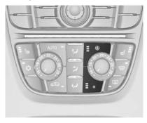
Press lower button to decrease or upper button to increase fan speed as shown in the illustration. The fan speed is indicated by the number of segments in the display.
