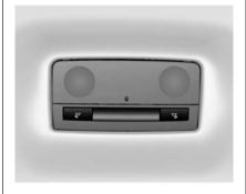
Illuminates in conjunction with the front courtesy light depending on rocker switch position.
