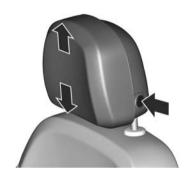
**Height adjustment**Press and hold button, adjust height, release button to engage.
