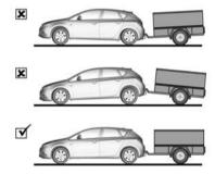
If the attitude of the vehicle is compromised, adjust the vehicle and trailer load within the specifications to improve the attitude. If the vehicle attitude cannot be corrected, use a load distribution hitch.
