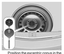
recess of the spare wheel before tightening the wing nut.
