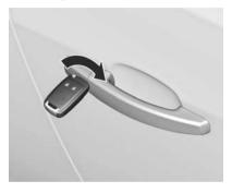
Manually unlock the driver's door by turning the key in the lock. Switch on the ignition and press the central locking button to unlock the other doors, tailgate and fuel filler flap.
