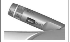
Press **MENU** to switch between the menus or to return from a submenu to the next higher menu level.
