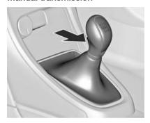
Reverse: with the vehicle stationary, wait 3 seconds after depressing clutch pedal and then press the release button on the selector lever and engage the gear.
