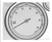
Displays the engine speed.
