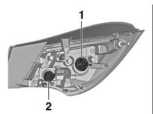
5. Remove the bulb holder by turning and replace the bulb by withdrawing or pushing the bulb slightly into the socket and rotating anticlockwise:
