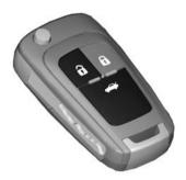
Press do to unlock the doors, tailgate and fuel filler flap. Open the doors by pulling the handles.
