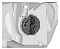
Rotate bulb socket (2) anticlockwise to disengage. Withdraw the bulb socket from the reflector.
