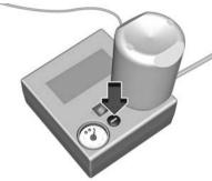
If the prescribed tyre pressure is not obtained within 10 minutes, remove the tyre repair kit. Move the vehicle one tyre rotation. Reattach the tyre repair kit and continue the filling procedure for 10 minutes.
