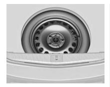
The spare wheel is located in the load compartment beneath the floor covering. It is secured with a wing nut. To remove:
