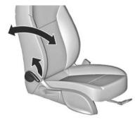
Pull lever, adjust inclination and release lever. Allow the backrest to engage audibly.
