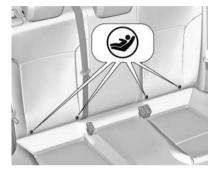
Fasten vehicle-approved ISOFIX child restraint systems to the ISOFIX mounting brackets. Specific vehicle ISOFIX child restraint system positions are marked in the table.
