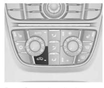
Press to activate the air recirculation mode. The LED in the button illuminates to indicate activation.
