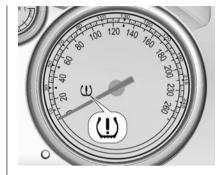
A detected low tyre pressure condition is indicated by illumination of control indicator (೨) ⇒ 71.
