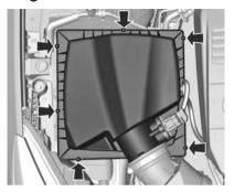
To replace engine air filter unscrew 6 screws and remove air filter housing.
