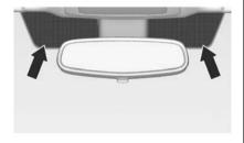
The marked areas on the windscreen are not covered with the coating. Devices for electronic data recording and fee payment must be attached in these areas. Otherwise data recording malfunctions may occur.
