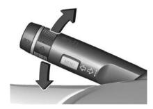
lever up : right turn signal lever down : left turn signal
