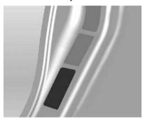
The identification plate is located on the front left door frame.
