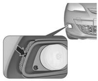
Disengage the cover with a screwdriver in the recess and remove the cover.
