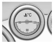
Displays the coolant temperature.
