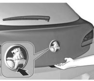
Press on radio remote control (if equipped) or push the brand emblem at the bottom half to unlock and open the tailgate.
