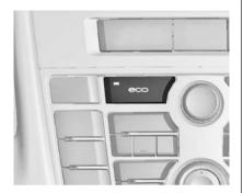
Deactivate the stop-start system manually by pressing **eco**.
