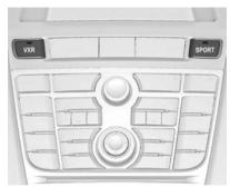
VXR Flex Ride driving system allows the driver to select between three driving modes:
