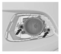
2. Unscrew both screws and remove light assembly from the bumper.
