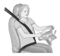
The seat belts are locked during hard acceleration or deceleration of the vehicle holding the occupants in the seated position. Therefore the risk of injury is considerably reduced.
