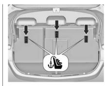
The fastening eyes are on the backside of rear seats.
