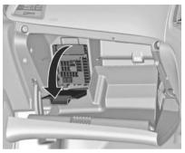
The fuse box is located behind a cover in the glovebox. Open the glovebox, then open the cover and fold it down.
