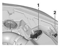
**Bi-Halogen Headlight (1)** with one bulb for low and high beam.
