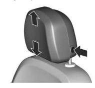
Press and hold button, adjust height, release button to engage.
