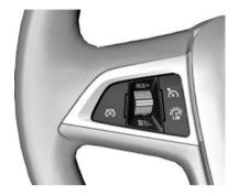
Press ②. If cruise control has been activated before, it is switched off when speed limiter is activated and the control indicator ③ extinguishes.
