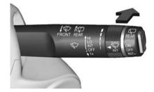
Push lever. Washer fluid is sprayed onto the rear window and the wiper wipes a few times.
