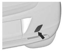
Insert a screwdriver in the slot at the lower bend of the cap. Release the cap by carefully moving the screwdriver downwards.
