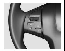
The infotainment system can be operated by the controls on the steering wheel.
