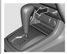
**P**: (park) In park position, the wheels are locked. Select **P** only when the vehicle is stationary and the parking brake is applied.
