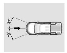
Front airbags will inflate in certain severe frontal or near frontal impacts. Front airbags are not designed to inflate if the vehicle is struck from the side, rear or in rollovers. Always wear a seat belt.
