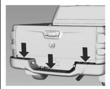
The maximum load on the rear bumper is 100 kg.
