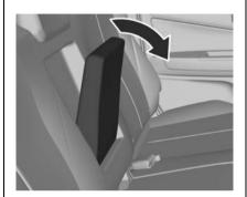
Unfold the armrest by pulling downwards from the top.
