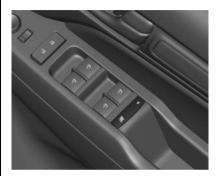
Press switch to deactivate the power windows of the rear doors. The other power windows can be operated by switches on the driver's door.
