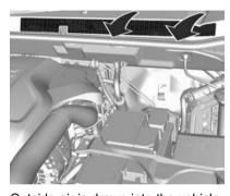
Outside air is drawn into the vehicle through the opening between the bonnet and the windscreen.
