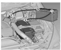
Connect one end of the red lead to the positive terminal of the booster battery (1).
