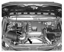
Pull the support rod up and away from the holder and secure.
