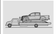
A flat-bed tow truck is the best method of towing the vehicle to avoid damage.
