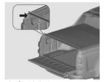
Stretch the tonneau cover on the load compartment, fitting the rear beam in to the side rail support without locking it.
