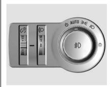
When the automatic light function **AUTO** is switched on, the system switches on the headlights and taillights automatically, depending on the exterior illumination conditions.
