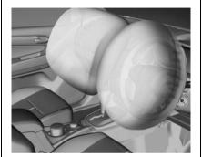
The front airbag system consists of one airbag in the steering wheel, one in the instrument panel on the passenger's side and a knee airbag in the lower part of the driver's side instrument panel.
