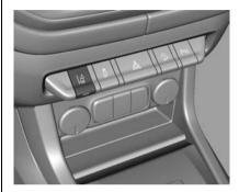
If equipped, LDW may help avoid crashes due to unintentional lane departures. It may provide an alert if the vehicle is crossing a lane without using a turn signal in that direction. LDW uses a camera to detect the lane markings at speeds of 60 km/h or greater.
