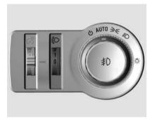
To set the headlight range according to vehicle load, turn the knob to the required position.
