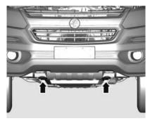
The vehicle may be recovered using the front towing eyes.
