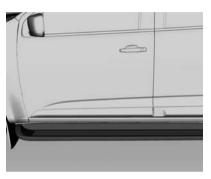
The side steps provide an extra foothold for accessing the front or rear doors.
