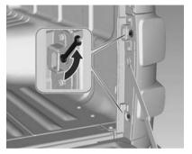
1. Unscrew both fasteners.
