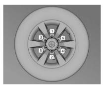
26. With the wheel on the ground, use the wheel wrench to tighten the wheel nuts in a crosswise sequence.
