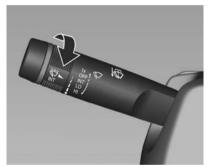
During intermittent operation, adjust the wiper interval:
