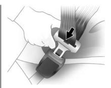
Loose or bulky clothing hinders the belt from fitting snugly. Do not place objects such as handbags or mobile phones between the belt and your body.
