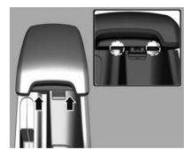
The armrest has a conduit for an auxiliary cable.
