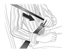
Withdraw the belt from the reel, guide it untwisted across the body and push the latch plate into the buckle until it clicks. Tension the lap belt regularly while driving by tugging the shoulder belt.
