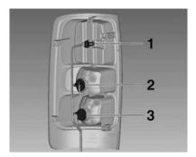
For LED version just replace lights 2 and 3. The brake light should be replaced by a Holden dealer.
