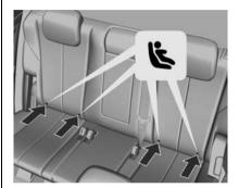
Fasten vehicle-approved ISOFIX child restraint systems to the ISOFIX mounting brackets.
