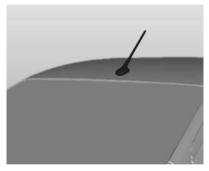
To remove the roof antenna, rotate it anticlockwise. To install the roof antenna, rotate it clockwise.
