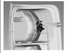
4. Rotate the relevant bulb holder counterclockwise.
