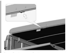
In order to open the tonneau cover, lower the tailgate and pull the release lever on the underside of the tonneau cover down.
