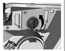
Rotate bulb holder counterclockwise and disengage.
