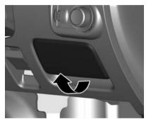
Remove the instrument panel cap in the direction of the arrow.
