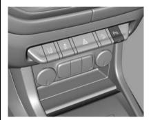
The P™ button of the instrument panel is used to turn on or off the Front and Rear Parking Assist. The indicator LED next to the button comes on when the features are on and turns off when the features have been disabled.
