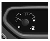
Shows the level of fuel in the tank. If the fuel level is low:
