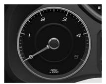
Shows engine speed in thousands of revolutions per minute (RPM).
