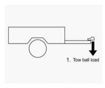
A trailer hitched to a vehicle places a weight on the tow bar. This weight is called the tow bar ball weight or tow ball load (1).
