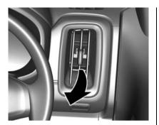
Direct the air flow by tilting and swivelling the adjuster knob.
