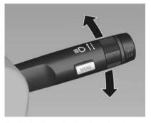
Push the lever in the direction the steering wheel is turned.
