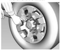
Turn the wheel wrench anticlockwise to loosen all the wheel nuts.
