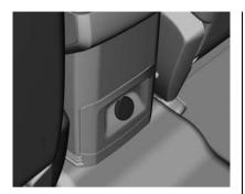
A 12V power outlet may be located on the back of the front center console.
