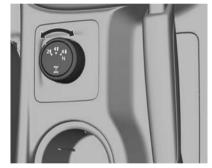
Rotate the shift control switch to shift into and out of four-wheel drive. You can choose from the following:
