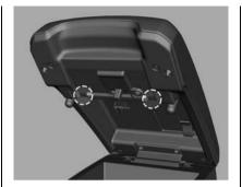
Use the conduit shown above to prevent pinching the auxiliary cable when the console armrest is down and the cable is in use.
