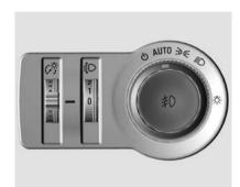
The front fog lamps provide extra illumination to the sides of the road and improve visibility in fog or snow.
