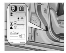
The correct pressures for tyres are shown on the tyre placard in the driver's door frame and in the tyre pressure table. See *Tyre Pressure* ⇒ 272.
