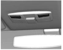
1. Press the button to turn the lamp on.
