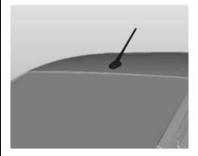
To remove the roof antenna, rotate it anticlockwise. To install the roof antenna, rotate it clockwise.
