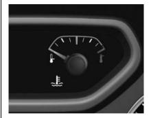
Shows the engine coolant temperature.
