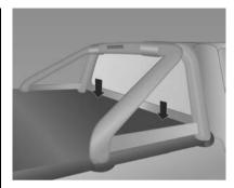
Push down along the front edge of the cover until it is secure.
