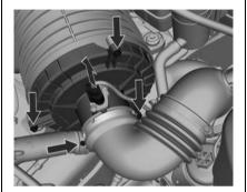
To replace the engine air filter, release the clamp and remove the air cleaner outlet duct. Disconnect the air sensor, unscrew the 3 screws and remove the filter housing.
