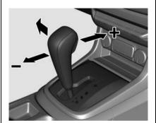
Move the selector lever out of position **D** towards the left and then forwards or backwards as desired.
