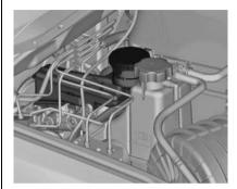
The level should be between the **MIN** and **MAX** marks.
