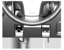
1. Pull the release lever rearwards and upwards.
