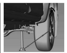
If the flat tyre is on the rear, position the jack under the rear axle as close as possible to the shock absorber (2).
