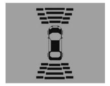
The instrument cluster may have a parking assist display with bars that show "distance to object" and object
