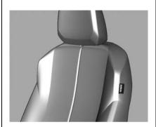
The vehicle may have Side Impact Airbags (SIAB) that are stored in the sides of the front seats, the side closest to the door.
