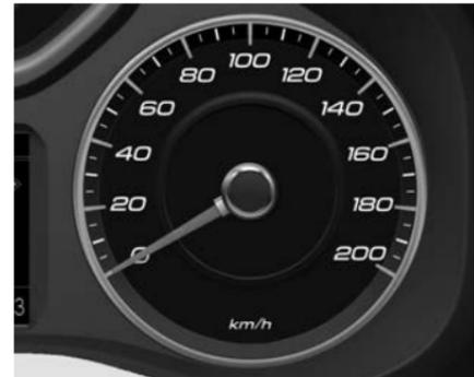
Shows vehicle speed in kilometres per hour (km/h).
