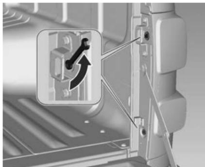
1. Unscrew both fasteners.
