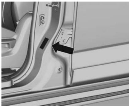
A label containing the vehicle build date is also located on the front passenger's door frame or on the rear door frame (Space Cab).
