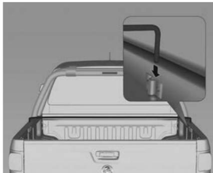
1. Slide the bow through the tonneau bow support bracket.
