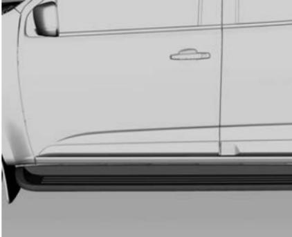
The vehicle may have side steps which provide an extra foothold for accessing the front or rear doors (if applicable).
