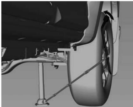
If the flat tyre is on the rear, position the jack under the rear axle as close as possible to the shock absorber (2).
