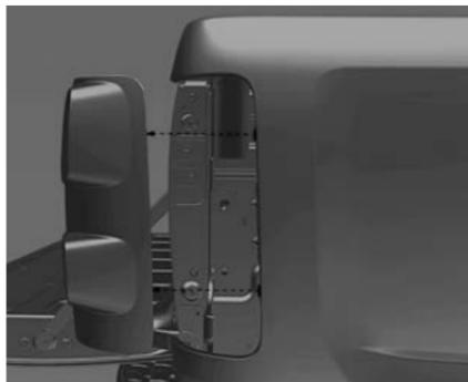
2. Remove the tail lamp assembly by pulling it straight out from the body. Take care that the cable duct remains in position.
