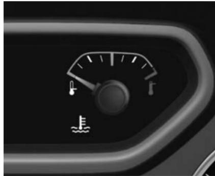
Shows the engine coolant temperature.
