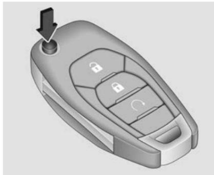
1. Press the button to extend the key blade.
