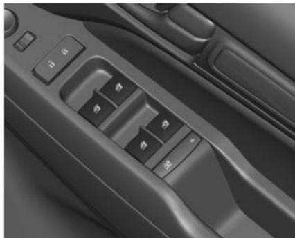
Operate the switch for each respective window by pushing to open, or pulling to close. The driver's window switch incorporates a light which signals operating readiness when illuminated.
