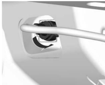
2. From the rear side of the bumper, rotate the bulb holder anticlockwise to disengage.
