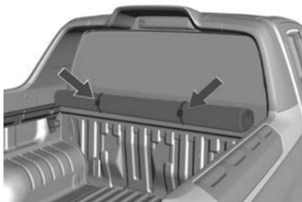
If you use the load compartment with the tonneau cover open, first roll up the tonneau cover and then secure with the straps.
