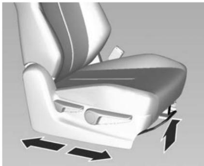
1. Move the seat forwards or backwards by lifting the handle at the front and sliding the seat.
