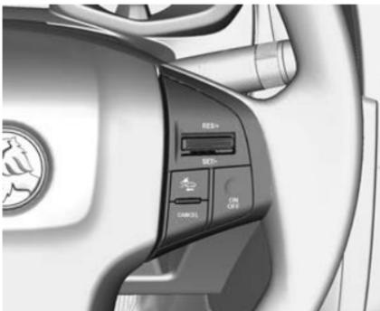
The Cruise Control and the Forward Collision Alert can be operated by the controls on the steering wheel.
