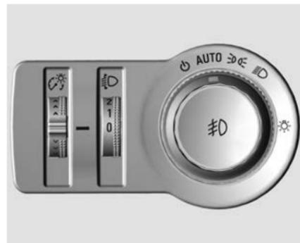
When the exterior lamp control switch is set to **AUTO**, the system automatically turns the headlamps and tail lamps on, depending on the exterior illumination conditions.
