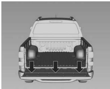
To avoid damage to the tailgate, limit the load placed on it:
