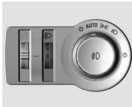
To set the headlamp level according to vehicle load, turn the dial to the required position.
