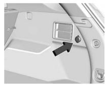
A 12V power outlet is also located in the rear load compartment.
