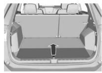
2. Fold the rear part of the load floor to the front.
