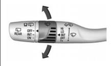
**INT:** Intermittent wipes. Turn the band up for more frequent wipes or down for less frequent wipes.
