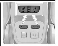
If equipped, the rear heated seat controls are on the rear of the centre console. To operate, the engine must be running.
