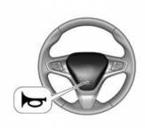
Press on the steering wheel pad to sound the horn.
