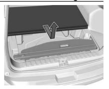
If desired, pull the load floor rearward slightly to disengage the retaining clips, and then lift upward to remove.
