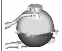
Check the coolant level in the coolant surge tank when the engine is cold.
