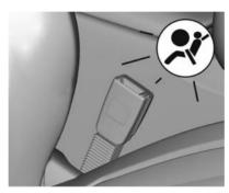
Front seat belt pretensioners are part of the SRS. In certain severe collisions the seat belts are tightened by the seat belt pretensioners.
