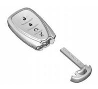
Press the button on the side of the RKE transmitter and remove the mechanical key.
