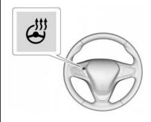
If equipped with a heated steering wheel, press to turn on or off. A light near the button displays when the feature is turned on.
