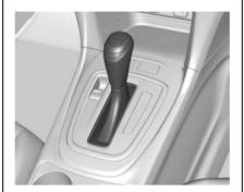
Press the select button on the front of the shift lever to move into any position. The lever position is displayed in the Driver Information Centre (DIC).
