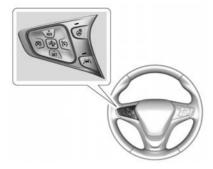
To turn LKA on and off, press and hold from the steering wheel.
