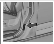
The correct pressures for tyres are shown on the tyre placard on the front passenger door frame and also in the tyre pressure table. See *Tyre Pressure* \$322.
