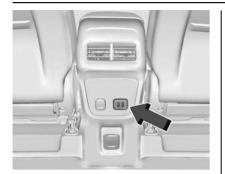
A USB port may also be located at the rear of the centre console. This port is for charging USB devices only.
