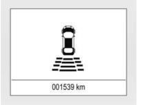
Additionally, the distance to rear objects is displayed by changing distance lines in the Driver Information Centre (DIC). The distance indication can be inhibited by vehicle messages with a higher priority. After dismissing the message, distance indication appears again.
