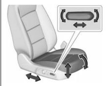
To adjust a power driver seat, if equipped:
