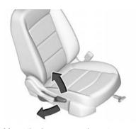
Move the lever up or down to manually raise or lower the seat.
