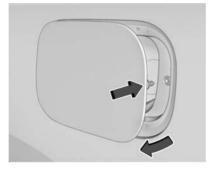
The fuel cap is behind the fuel door on the passenger side of the vehicle.
