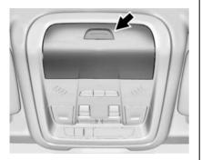
A covered storage compartment for sunglasses is located in the overhead console. Press the latch to open.
