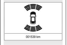
Additionally, the distance to rear and front obstacles is displayed by changing distance lines in the DIC.
