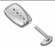
Remove the mechanical key by pressing the button on the side of the RKE transmitter near the bottom and pull the key out. Never pull the key out without pressing the button.
