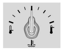
This gauge shows the engine coolant temperature when the ignition is on. Up level shown, mid level is similar.
