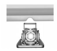
Locate the notch on the sheet metal weld flange. Place the centre of the jack lift head on the centre of the sheet metal notch.
