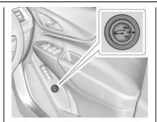
Choose the power liftgate mode by turning the dial on the switch to either the 3/4 or MAX position.
