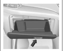
Open the glove box by lifting the lever.
