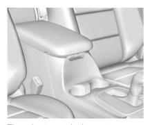
There is storage in the centre console; lift the lever on the front to open.
