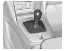
Select reverse gear while the vehicle is stationary.
