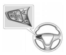
FCA can be disabled using the steering wheel control ⇒, or through vehicle personalisation.
