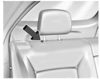
To lower the head restraint, press the button located on the top of the seat back, and push the head restraint down. Try to move the head restraint after the button is released to ensure it is locked in place.
