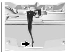
Go to the front of the vehicle and find the secondary bonnet release handle under the front edge of the bonnet near the centre.
