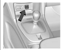
The front 12V power outlet is located in the centre console, below the climate control system.
