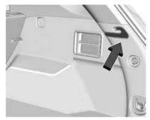
Engage the cover into the rear recesses in the side trims on each side.
