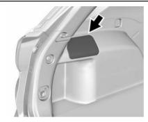
To access the fuse panel, carefully release the upper edge and remove the trim plate.
