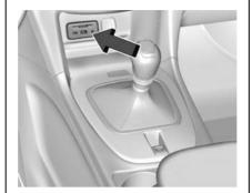
The vehicle has an auxiliary input jack located at the front of the centre console. Possible auxiliary audio sources include:
