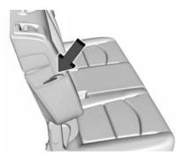
Remove the guide from its storage pocket on the side of the seat back
