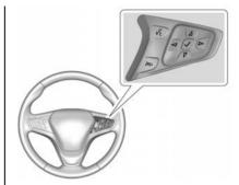
Press  $\triangleleft$  or  $\triangleright$  to select the DIC  $\bigcirc$  (Vehicle) page, then use  $\triangle$  or  $\bigcirc$  to scroll through the items to select Traction & Stability.
