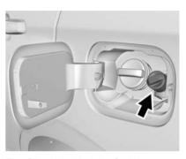
The filler is behind the fuel door next to the regular fuel cap. It has a blue cap.
