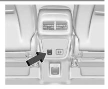
A 12V power outlet is also located at the rear of the centre console.
