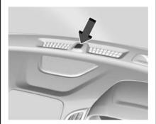
The indicator light, on the instrument panel near the windscreen, indicates the status of the system:
