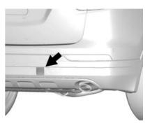
Carefully open the cover by using the small notch.
