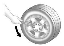
Turn the wheel wrench anticlockwise to loosen all the wheel nuts. Do not remove them yet.
