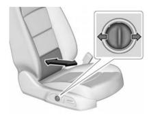
If equipped, press and hold the control switch forward or rearward to increase or decrease lumbar support.
