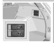
If equipped, the rear seat backs can also be folded forward by pulling the levers on the driver side of the rear cargo area.
