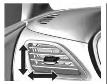
Direct the air flow by tilting and swivelling the slats.
