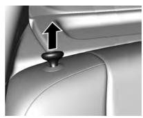
Pull the release knob on top of the rear seatback upwards.
