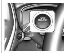
Electronic key must be inside the vehicle.
