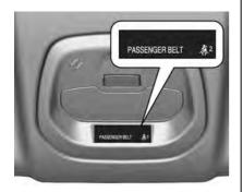
The front passenger's seat belt reminder displays (if occupied).
