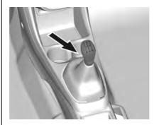
Reverse: with the vehicle stationary, press clutch pedal and engage the gear.
