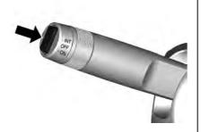
To operate the rear window wiper, push the switch at the end of the lever.
