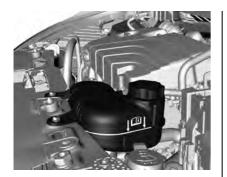
If the cooling system is cold, the coolant level should be above the line on the coolant reservoir.
