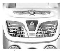
Press to turn the hazard warning flasher on or off, when the ignition is in any position.
