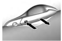
Electronic key system: Unlocking the vehicle by pressing the button on a front door handle deactivates the anti-theft system. The system is not deactivated when unlocking the driver's door with the key or with the central locking button in the passenger compartment.
