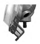
Reinstall the bulb holder into the lamp and rotate it clockwise until the centre of the bulb holder is placed at the arrow shape on the lamp.
