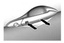
Press the button on either front door handle. The doors and tailgate are unlocked.
