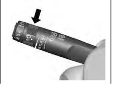
During intermittent operation, adjust the wiper interval:
