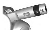
Rotate the adjuster wheel  $\stackrel{\triangle}{\nabla}$  to select the trip computer mode.
