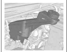
Check the brake fluid level weekly.
