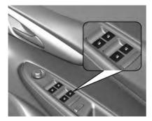
The power windows can be operated when the ignition is on.
