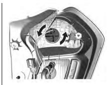
3. Rotate the applicable bulb holder anticlockwise.
