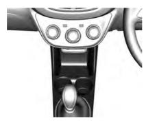
The instrument panel storage compartment is located in front of the shift lever.
