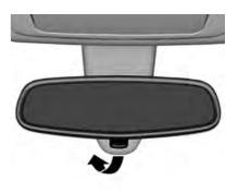
To reduce headlamp glare from following vehicles, push the lever towards the front of the vehicle.
