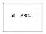
Estimates driving distance to an empty fuel tank from the current fuel level.
