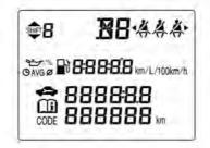
The Driver Information Centre (DIC) is located in the instrument cluster. The DIC displays functions such as the trip computer, information and warning messages and settings, etc.
