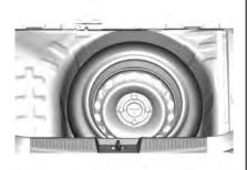
The spare tyre is located in the load compartment beneath the floor covering.
