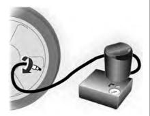
13. Unscrew the valve cap from the defective tyre.
