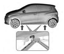
Position the jack beneath the jack location closest to the wheel being changed.
