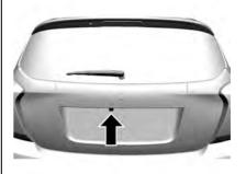
The camera is located on the tailgate at the rear of the vehicle.
