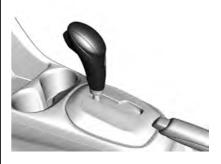
**P**: (park) In park position, the front wheels are locked. Select P only when the vehicle is stationary and the parking brake is applied.
