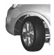
Turn the front wheels and remove 2 push nuts on outside of wheel liner.
