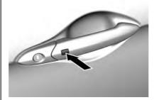
Press the button on either front door handle. The doors and tailgate are locked.
