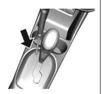
Insert a flat-blade screwdriver into the opening as far as it will go and move the shift lever out of P (park).
