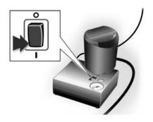
15. Press the switch on the compressor to I.
