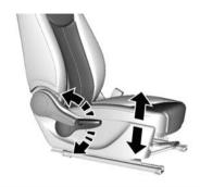
Pump the lever on the outside of the seat cushion.
