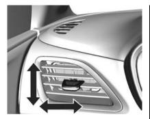
Direct the air flow by tilting the slats.
