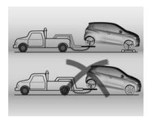
Alternatively, use a standard tow truck and a towing dolly to prevent the front wheels from contacting the road.
