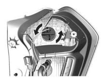
3. Rotate the applicable bulb holder anticlockwise.
