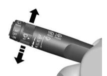
To operate the windscreen wipers, turn the ignition on and move the windscreen wiper/washer lever up or down to the desired position.
