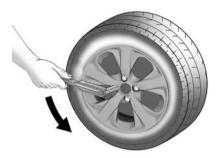
Place the wheel wrench over the wheel nuts and loosen by half a turn, but do not remove the wheel nuts.
