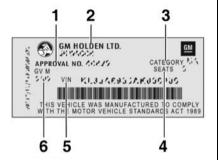
An identification and compliance label is located on the front passenger door frame.
