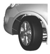
Turn the front wheels and remove 2 push nuts on outside of wheel liner.
