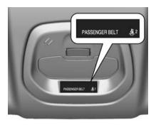
The front passenger's seat belt reminder displays (if occupied).
