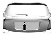
The camera is located on the tailgate at the rear of the vehicle.
