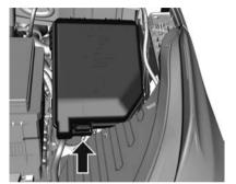
1. To disengage the cover, lift upwards and remove.
