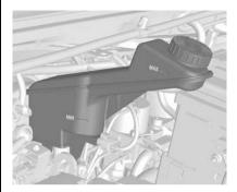
Check the brake fluid level weekly.
