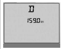
The top line displays the recorded distance since the last reset.
