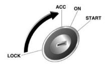
**LOCK**: When the key is in this position, some electrical accessories and the engine are off.
