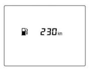
Estimates driving distance to an empty fuel tank from the current fuel level.
