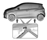
Position the jack beneath the jack location closest to the wheel being changed.
