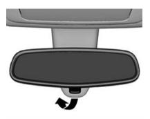
To reduce headlamp glare from following vehicles, push the lever towards the front of the vehicle.
