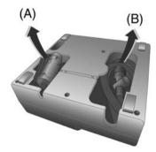
Remove the electrical connection cable (A) and air hose (B) on the underside of the compressor.
