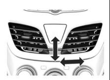
Direct the air flow by tilting the slats. The centre vents cannot be closed.
