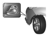
Turn the front wheels and remove 2 push nuts on outside of wheel liner.
