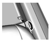
2. Pull the fuel filler door release lever up.
