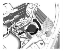
1. Rotate the washer funnel anticlockwise to disengage.
