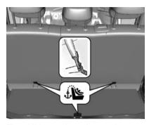
The child restraint tether anchors are located on the backside of the rear seats and the centre of the rear end panel at the load compartment area.
