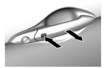
Electronic key system: Unlocking the vehicle by pressing the button on a front door handle deactivates the anti-theft system. The system is not deactivated when unlocking the driver's door with the key or with the central locking button in the passenger compartment.
