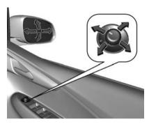
Select the relevant exterior mirror by turning the control left (L) or right (R). Then swivel the control to adjust the mirror. In position 0 no mirror is selected.
