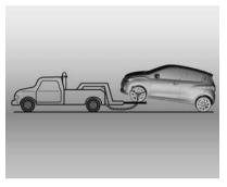
Use a standard tow truck, where the front wheels are raised and the rear wheels are in contact with the ground.
