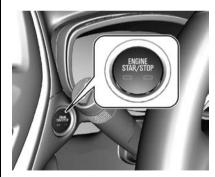
Electronic key must be inside the vehicle.
