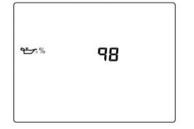
Displays an estimate of the remaining useful oil life. This may only be displayed while the vehicle is stationary.
