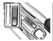
Place the electronic key in the centre console transmitter pocket. Press the brake pedal and press the Engine Start/Stop button.
