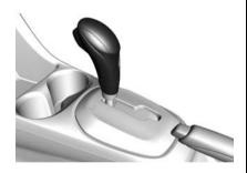
**P**: (park) In park position, the front wheels are locked. Select P only when the vehicle is stationary and the parking brake is applied.
