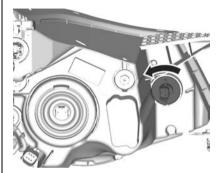
1. Rotate the bulb holder anticlockwise to disengage.
