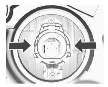
7. Press the spring clip to disengage.
