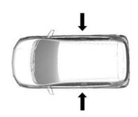
The curtain airbags deploy in most, but not all severe side impacts.
