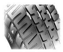
Replace the tyres when they are worn to the point where the tread wear indicators (TWI) appear.
