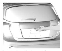
To open the tailgate, push the touchpad switch under the tailgate moulding.
