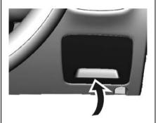
The interior fuse box is located on the underside of the driver side of the instrument panel.
