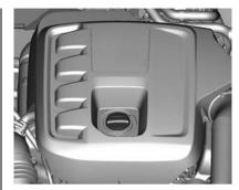
The engine oil filler cap is located on the top of the engine.
