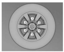
27. With the wheel on the ground, use the wheel wrench to tighten the wheel nuts in a crosswise sequence.
