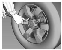
16. Turn the wheel wrench anticlockwise to loosen all the wheel nuts.
