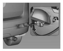
Behind the rear bumper, unscrew the screw to remove the reverse lamp assembly and disconnect the electrical connector.
