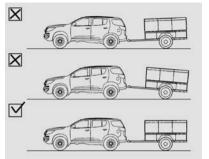
For single-axle trailers, the tow ball load should be 10 % of the loaded trailer weight. For heavy trailers with more than one axle, the tow ball load should be 5 % -10 % of the loaded trailer weight.
