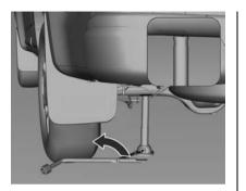
When positioning the jack under the rear axle housing, confirm that the slot on the upper side of the jack fits on the axle.
