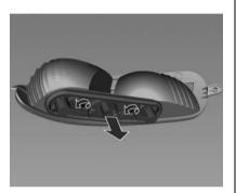
2. Unscrew the both screws to remove the bulb holder.
