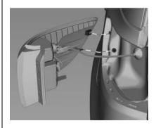
2. Remove the tail light assembly by pulling straight out of the body. Remove the electrical connector.
