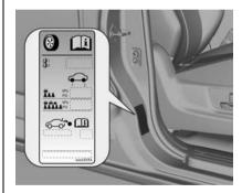
The correct pressures for tyres are shown on the tyre placard in the driver's door frame and in the tyre pressure table. See *Tyre Pressure*  $\Rightarrow$  278.
