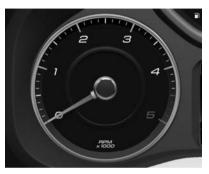
Shows engine speed in thousands of revolutions per minute (RPM).
