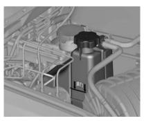
If the cooling system is cold, the coolant level should be above the line on the coolant reservoir.
