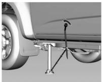
If the flat tyre is on the front of the vehicle, position the jack to the rear of the front tyre in the cut out on the frame (1).
