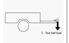
A trailer hitched to a vehicle places a weight on the tow bar. This weight is called the tow bar ball weight or tow ball load (1).
