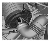
To replace the engine air filter, release the clamp and remove the air cleaner outlet duct. Disconnect the air sensor, unscrew the 3 screws and remove the filter housing.
