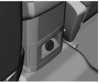
The 12V power outlets are located in front of the shift lever and at the rear of the centre console.
