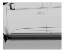
The side steps provide an extra foothold for accessing the front or rear doors.
