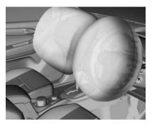
The front airbag system consists of one airbag in the steering wheel, one in the instrument panel on the passenger's side and a knee airbag in the lower part of the driver's side instrument panel.
