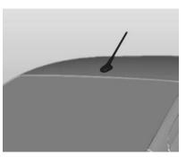
To remove the roof antenna, rotate it anticlockwise. To install the roof antenna, rotate it clockwise.
