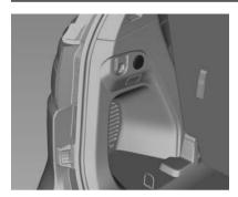
A power outlet is located on the passenger side of the load compartment.
