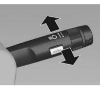
To switch from low to high beam, push the lever.
