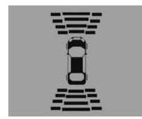
The instrument cluster may have a parking assist display with bars that show "distance to object" and object
