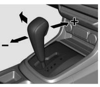
Move the selector lever out of position **D** towards the left and then forwards or backwards as desired.
