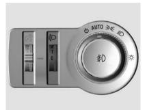
To set the headlight range according to vehicle load, turn the knob to the required position.
