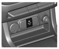
The rear air conditioning system is operated with the **REAR A/C** button.
