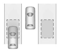
The SBZA sensor covers a zone of approximately one lane over from both sides of the vehicle, or approximately 3.5 m. The height of the zone is approximately between 0.5 m and 2 m off the ground. This zone starts at approximately the middle of the vehicle and goes back 5 m.
