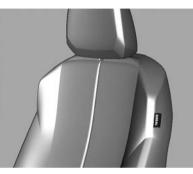
Side Impact Airbags (SIAB) are stored in the sides of the front seats, the side closest to the door.
