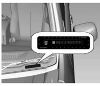
The VIN is also located on the instrument panel visible through the windscreen.
