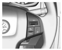
The Collision Alert control is on the steering wheel. Press  $\stackrel{\checkmark}{\rightarrow} \stackrel{\frown}{\cong}$  to set the FCA timing to far, medium, near,
