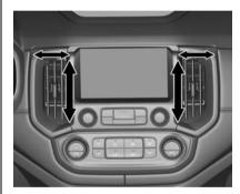
Push the slat up to open and down to close the vent or to adjust the air amount.
