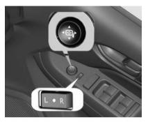
The control for the power mirrors are located on the driver's door.
