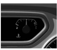
Shows the engine coolant temperature.
