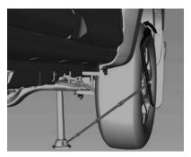
If the flat tyre is on the rear, position the jack under the rear axle and get as close as possible to the shock absorber (2).
