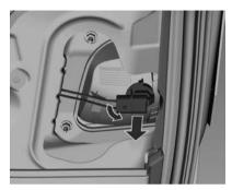
3. Rotate the relevant bulb holder anticlockwise and remove it.
