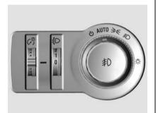
When the automatic light function **AUTO** is switched on, the system switches on the headlights and taillights automatically, depending on the exterior illumination conditions.
