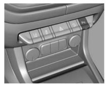
The P<sup>™</sup> button of the instrument panel is used to turn on or off the Front and Rear Parking Assist. The indicator LED next to the button comes on when the features are on and turns off when the features have been disabled.
