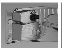
4. Rotate the relevant bulb holder counterclockwise.
