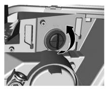
1. Rotate bulb holder counterclockwise and disengage.
