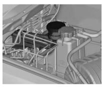
The level should be between the **MIN** and **MAX** marks.
