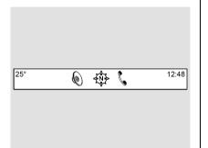
The applications tray is at the top-center of the screen. The applications tray can have three to five applications.
