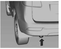
The vehicle may be recovered using the front or rear towing eyes.
