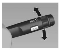
Push the lever in the direction the steering wheel is turned.
