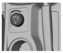
Rotate the shift control switch to shift into and out of four-wheel drive. You can choose from the following:
