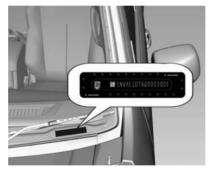
The VIN is also located on the instrument panel visible through the windscreen.
