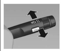
To switch from low to high beam, push the lever.
