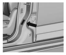
A label containing the vehicle built date is located on the front passenger's door frame.
