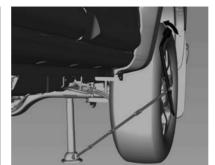
If the flat tyre is on the rear, position the jack under the rear axle and get as close as possible to the shock absorber (2).
