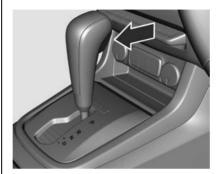
**P**: (park) In park position, the wheels are locked. Select **P** only when the vehicle is stationary and the parking brake is applied.
