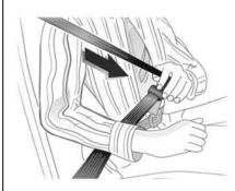
Withdraw the belt from the reel, guide it untwisted across the body and push the latch plate into the buckle until it clicks. Tension the lap belt regularly while driving by tugging the shoulder belt.
