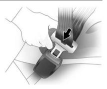
Loose or bulky clothing hinders the belt from fitting snugly. Do not place objects such as handbags or mobile phones between the belt and your body.
