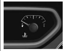
Shows the engine coolant temperature.
