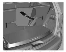
From the rear of the vehicle. pull the strap and release.
