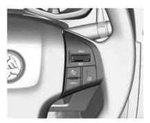
The Collision Alert control is on the steering wheel. Press to set the FCA timing to far, medium, near,
