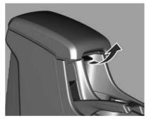
Press the latch and lift the armrest lid upward.
