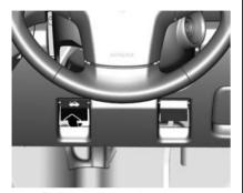
Pull the release lever rearwards and upwards.
