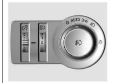
(b): With automatic light system, turn the switch to activate or deactivate the system, switch turns back to **AUTO**
