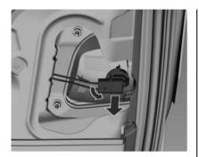
3. Rotate the relevant bulb holder anticlockwise and remove it.
