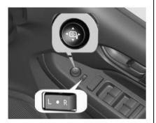
The control for the power mirrors are located on the driver's door.
