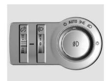
When the automatic light function **AUTO** is switched on, the system switches on the headlights and taillights automatically, depending on the exterior illumination conditions.
