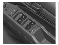
Operate the switch for each respective window by pushing to open or pulling to close. The switch for the driver's window has a light which signals, through illumination, the operation readiness.
