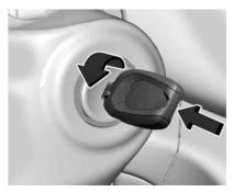
When the vehicle is stopped, push the key in toward the steering column and turn the key to Lock / Off to turn the engine off.
