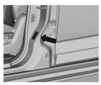
A label containing the vehicle build date is also located on the front passenger's door frame.
