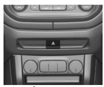
Press A to turn the hazard warning flasher on or off, when the ignition is in any position.
