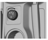
Rotate the transfer shift control switch to change the setting.
