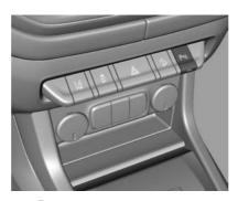
The P<sup>™</sup>▲ button of the instrument panel is used to turn on or off the front and rear parking assist. The indicator LED next to the button comes on when the features are on and turns off when the features have been disabled.
