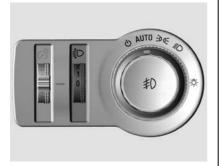
To set the headlamp level according to vehicle load, turn the dial to the required position. **0 or 1**: One person in the driver's seat, or both front seats occupied (2 passengers).
