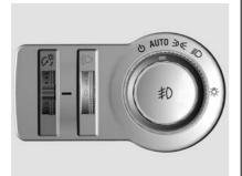
To adjust the instrument lighting brightness:
