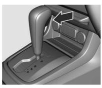
**P**: (park) In park position, the wheels are locked. Select **P** only when the vehicle is stationary and the parking brake is applied.
