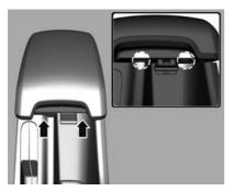
A USB and auxiliary port is located in the armrest storage compartment. To accommodate USB or auxiliary cable routing, recesses are provided.
