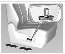
Move the seat forwards or backwards by sliding the switch.
