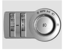
When the exterior lamp control switch is set to **AUTO**, the system automatically turns the headlamps and tail lamps on, depending on the exterior illumination conditions.
