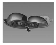
2. Unscrew the two screws to remove the bulb holder.
