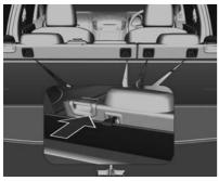
5. Push the cover forwards and engage it in the hooks on the back of the second row seats.
