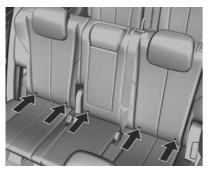
Fasten vehicle-approved ISOFIX child restraint systems to the ISOFIX mounting brackets.
