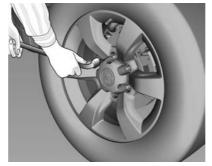
16. Turn the wheel wrench anticlockwise to loosen all the wheel nuts.
