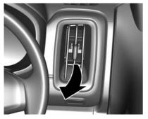
Direct the air flow by tilting and swivelling the adjuster knob.
