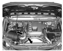
3. Remove the support rod from the holder and secure in the bonnet aperture.
