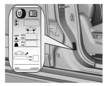
The correct pressures for tyres are shown on the tyre placard in the driver's door frame and in the tyre pressure table. See *Tyre Pressure* ⇔ 289.
