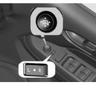
The controls for the power mirrors are located on the driver's door.
