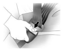
To release the belt, press the red button on the belt buckle.
