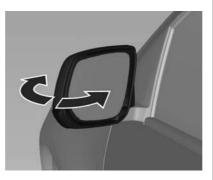
When the vehicle is parked, the mirrors may be folded flat against the side of the vehicle.
