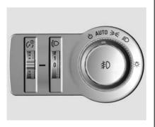
**AUTO :** Headlamps and exterior lamps are switched on and off automatically depending on external lighting conditions.
