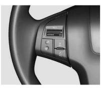
The infotainment system can be operated by the controls on the steering wheel.
