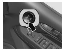
Press the selector switch (L / R switch) to the central position  $\bullet$ , then push the four-way switch down. Both exterior mirrors will fold.
