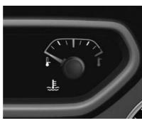
Shows the engine coolant temperature.
