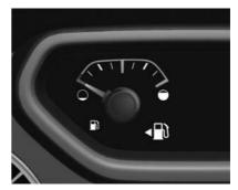
Shows the level of fuel in the tank.
