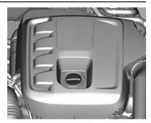
The engine oil filler cap is located on the top of the engine.
