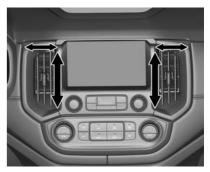
Push the adjuster knob up to open and down to close the vent or to adjust the volume of air.
