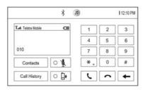
Touch son the screen or press on the steering wheel remote control. Alternately, press son the control panel.
