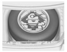
The jack and tools are located above the spare wheel, in the load compartment.
