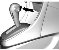
Movement between certain gear positions requires pressing the release button on the shift lever and/or depressing the brake pedal.
