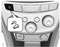
Press below 40 km/h. illuminates green on the instrument cluster indicating DCS is ready for use.
