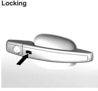
Press the button on the respective door handle. The doors, tailgate and fuel filler door are locked.
