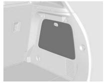
The tools and tyre repair kit are located in the load compartment on the driver's side.
