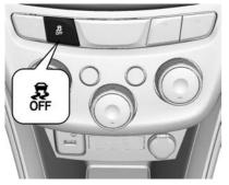
TCS can be deactivated when spinning of drive wheels is required:
