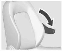
The vehicle may have an armrest on the driver's seat. It can be raised or lowered.
