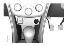
A 12V power outlet is located in the centre console.
