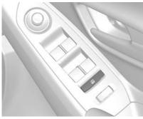
Press 🗷 to activate/deactivate the rear door power window switches.
