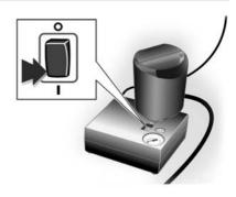
13. Press the switch on the compressor to **I**.
