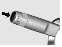
To operate the rear window wiper, push the switch at the end of the lever.
