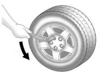
Place the wheel wrench over the wheel nuts and loosen by half a turn, but do not remove the wheel nuts.
