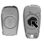
2. Remove the battery with a small tool by pushing it toward the top of the transmitter.
