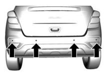
The PA system is able to detect and indicate obstacles at the rear of the vehicle when reversing.
