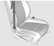
In the event of a front, side or rear collision of a certain severity, the driver's and/or passengers safety belts are tightened.
