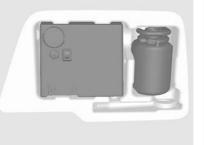
3. Remove the tyre repair kit from behind the cover in the load compartment, on the driver's side. 4. Remove the compressor and sealant bottle.
