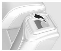
Pull the release lever on top of the rear seatback and fold it forwards and down.
