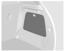
The vehicle may have an emergency tyre sealant and compressor kit, in place of a spare tyre. It is located in the load compartment on the driver's side.
