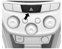
Press **A** to turn the hazard warning flashers on or off, when the ignition is in any position.
