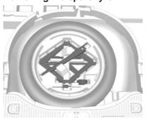
The spare tyre is located in the load compartment beneath the floor cover.
