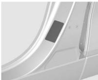
The correct pressures for tyres are shown on the tyre placard in the passenger's door frame.
