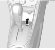
6. Remove the cap on the centre console with a thin object such as a flat-blade screwdriver.
